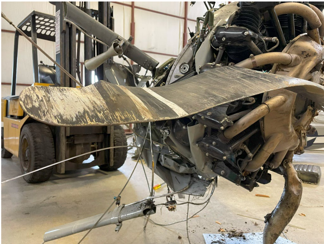
Figure 15. View of striations and S-bending.
