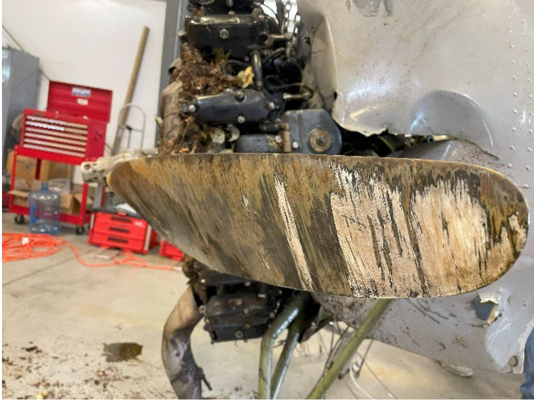
Figure 14. View of propeller blade striations.
