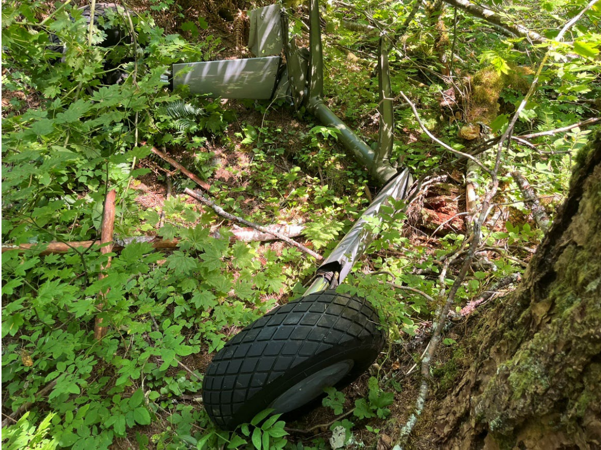
Figure 5. View of landing gear assembly (courtesy of FAA).
