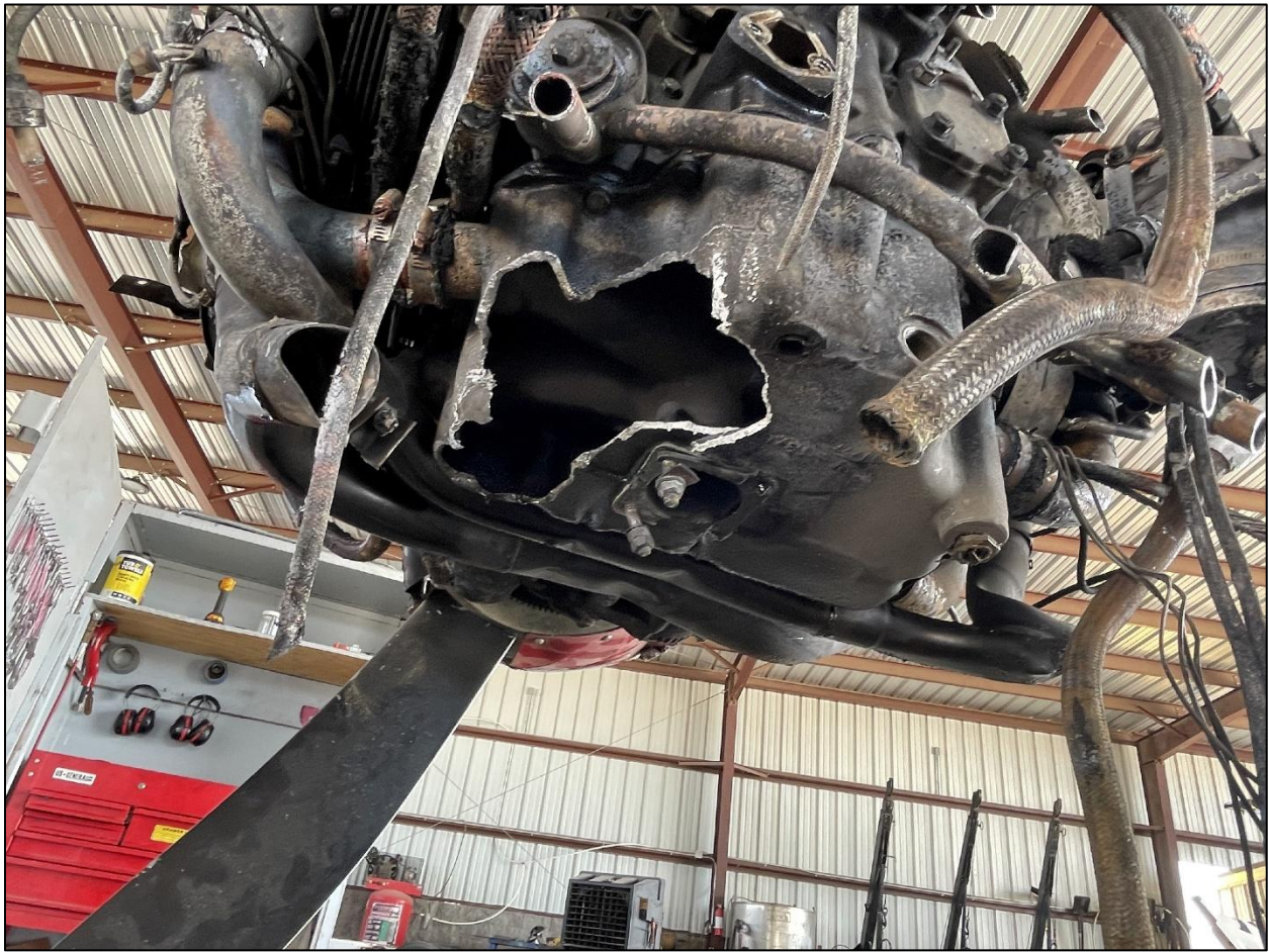
Figure 8-Engine oil sump damage.
