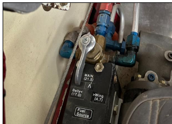
Figure 6-Fuel selector valve (preaccident), mounted left of the pilot's seat.
