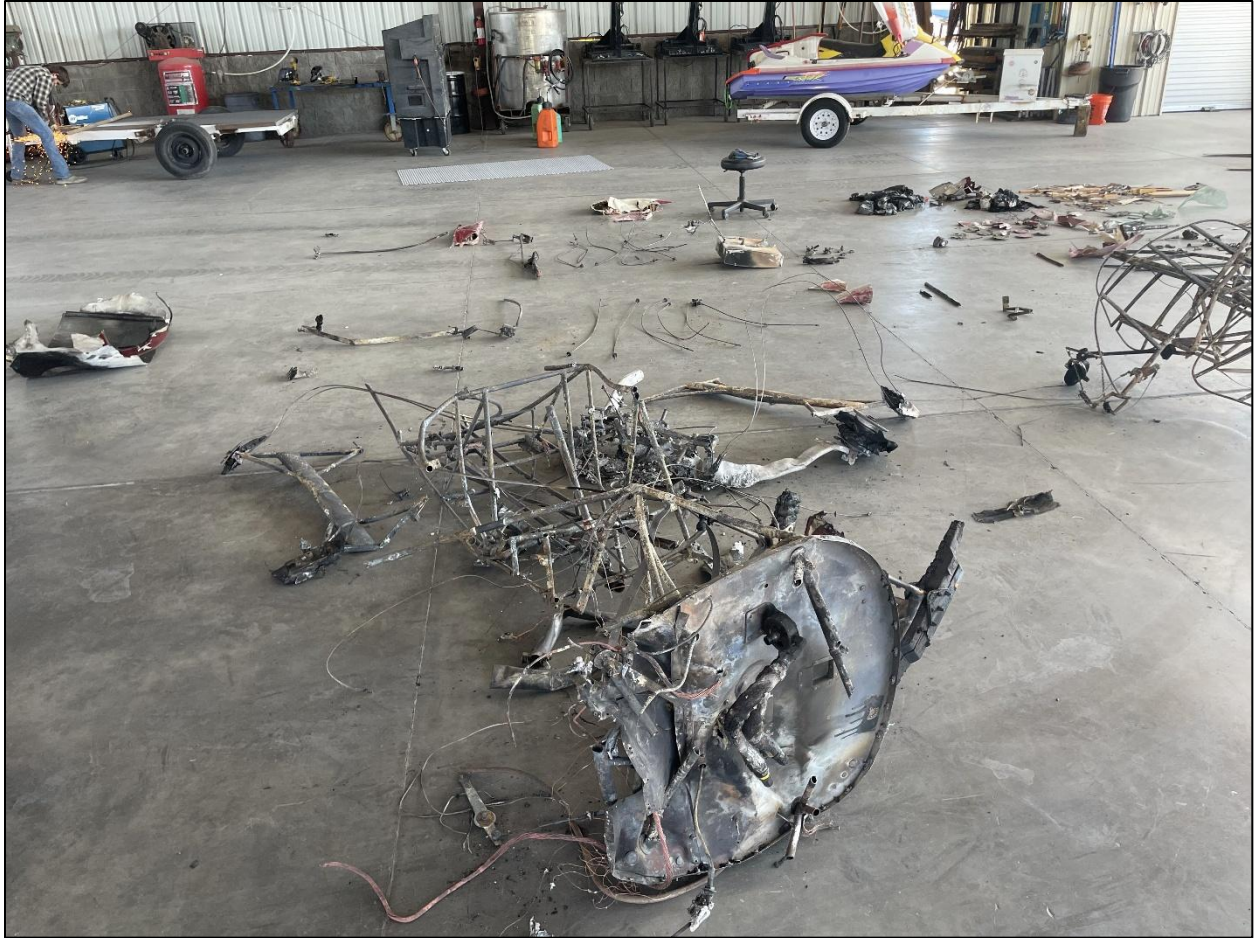
Figure 3-Wreckage layout, cabin area and forward fuselage structure.
