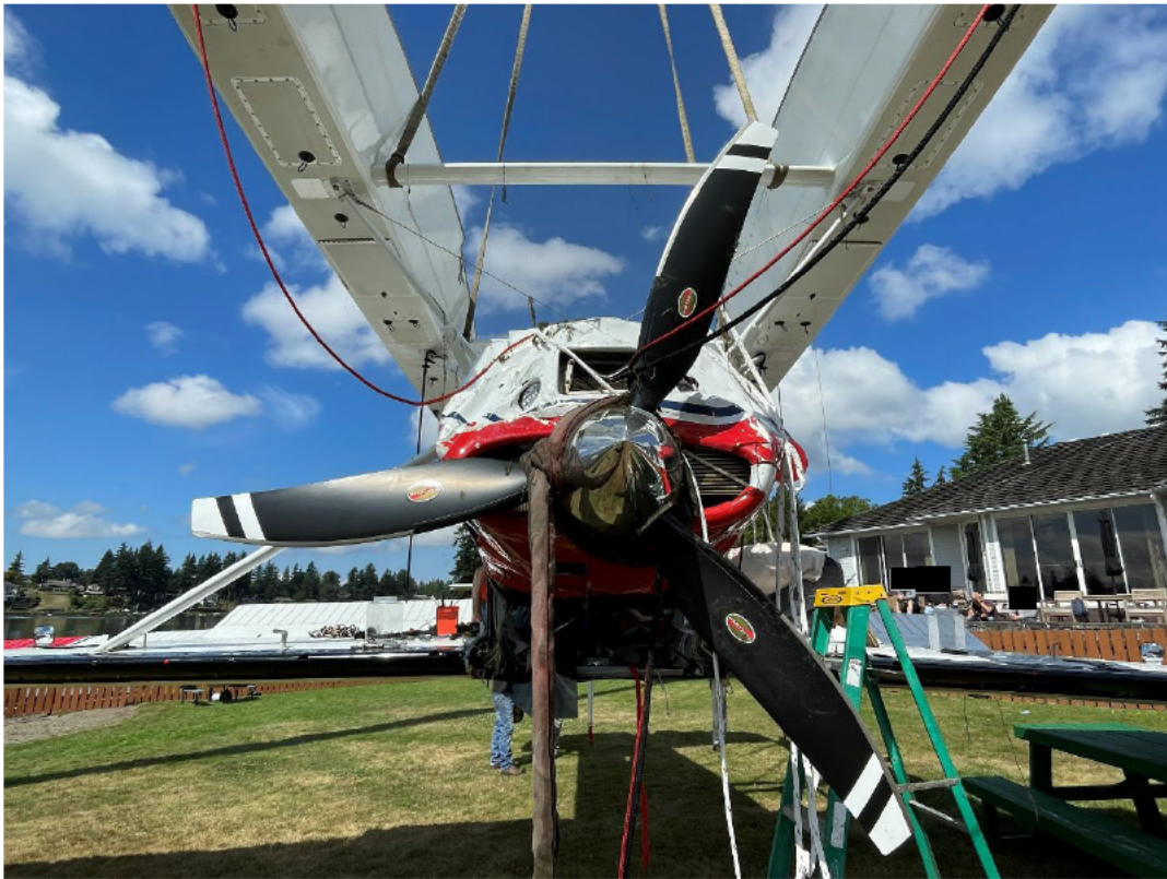
Figure 7. Propeller assembly during removal from lake.
