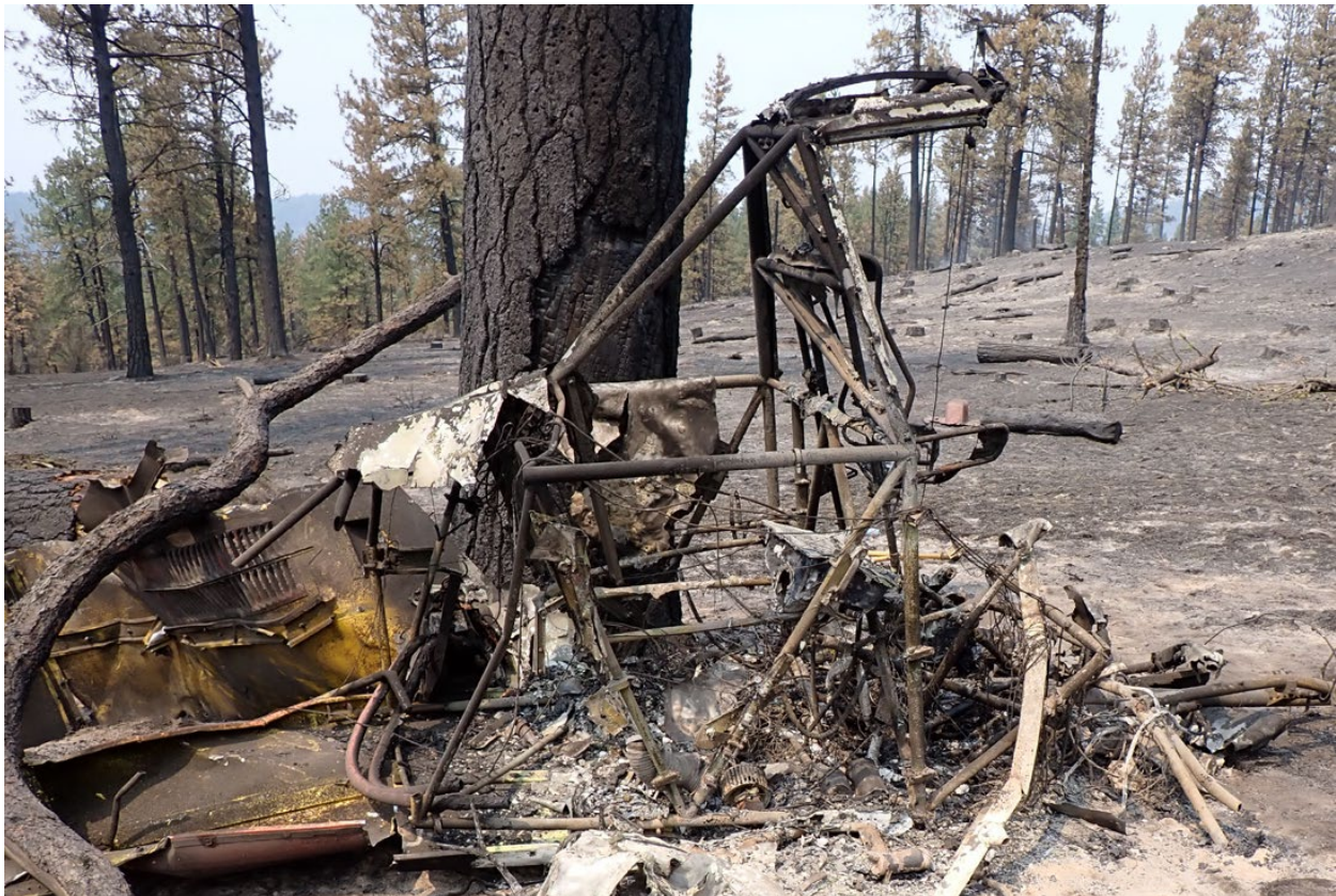
Figure 3. View of main fuselage resting against a tree
