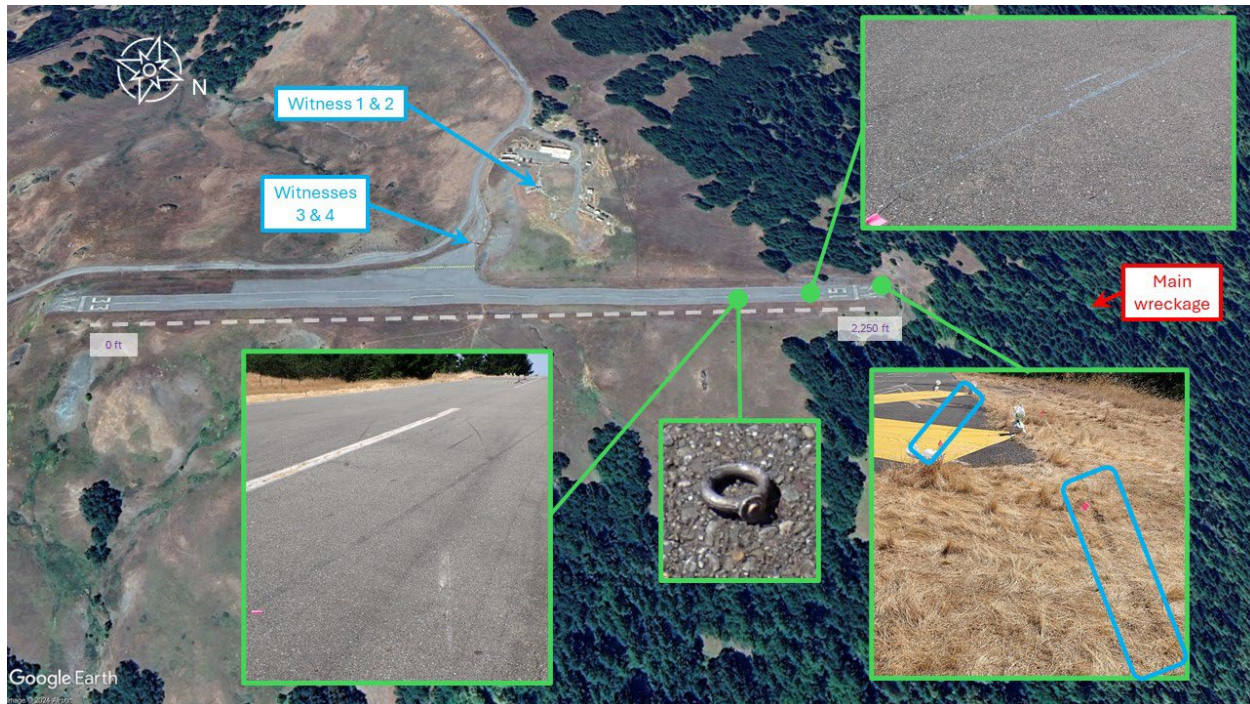
Figure 2: Images of runway contact signatures
