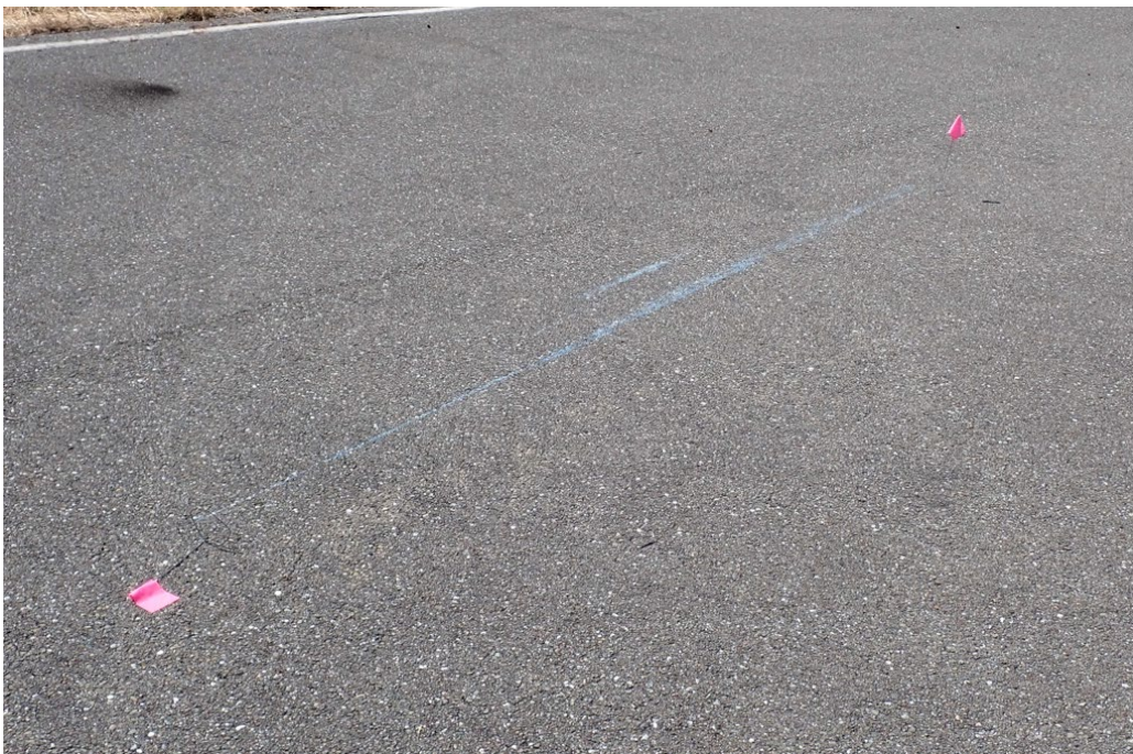
Figure 6: Blue runway contact marks
