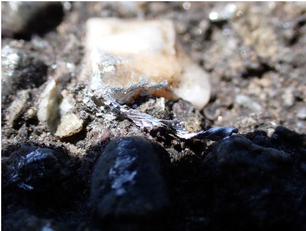
Figure 7: Metal fragment located next to blue contact marks
