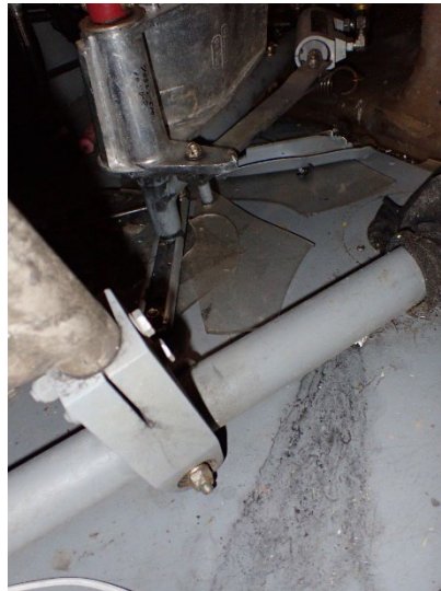
Figure 7. Control Stick Torque Tube (Photo Courtesy of Air Tractor)
