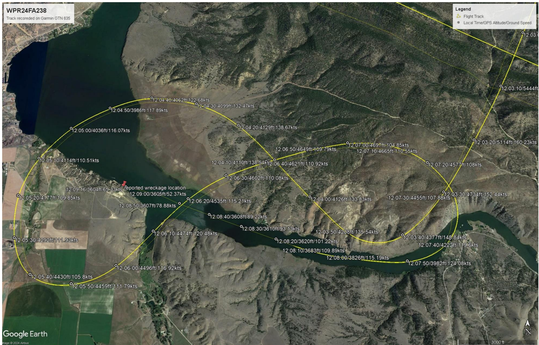
Figure 7. Google Earth overlay of the final seven minutes of the accident flight.
