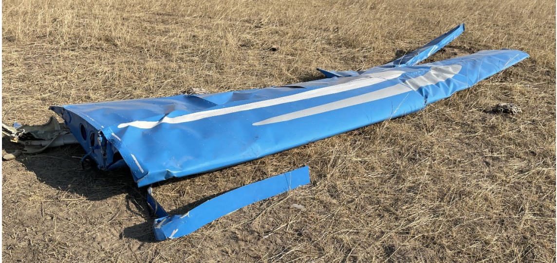
Figure 4: Front view left wing separated from fuselage.
