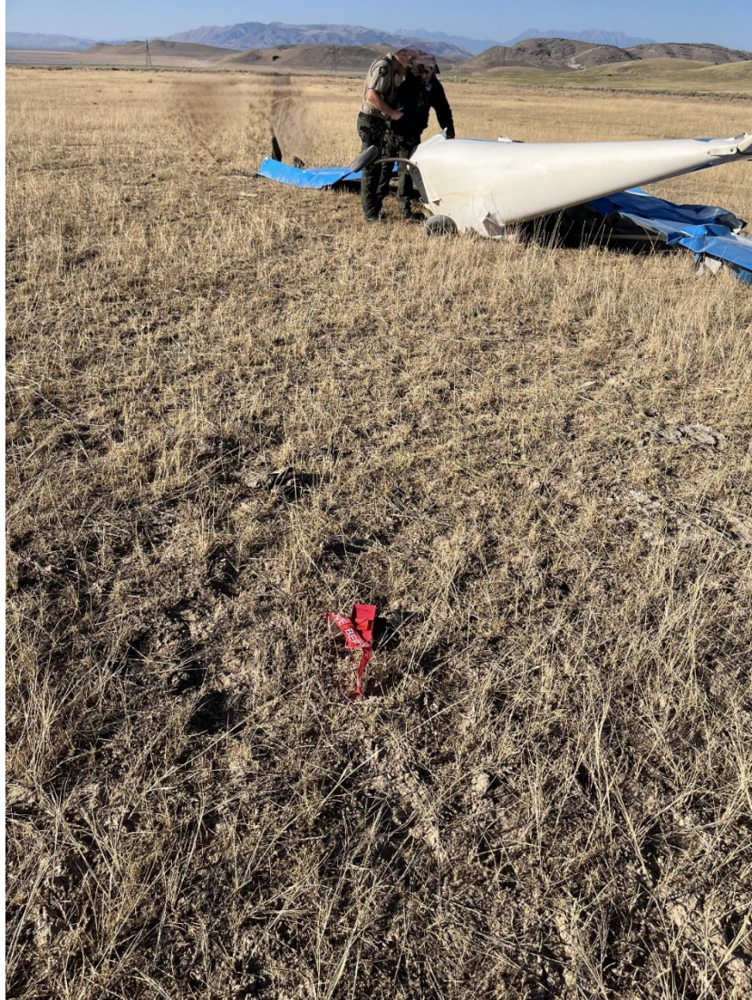
Figure 2: View of gust lock location on site (Courtesy of Utah Co Sheriff)
