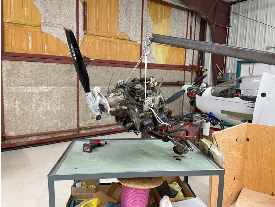
Figure 3 Engine with reduction gearbox attached
