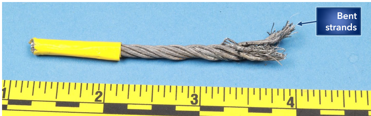
Figure 4. Fractured end of the cable after cutting and cleaning.
