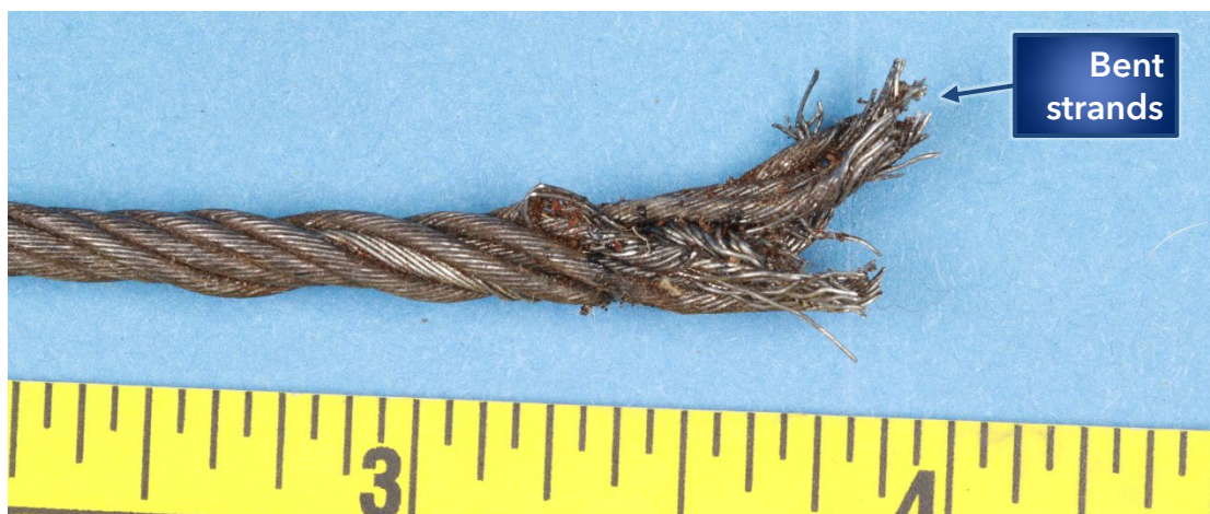
Figure 3. Fractured end after the tape was removed.
