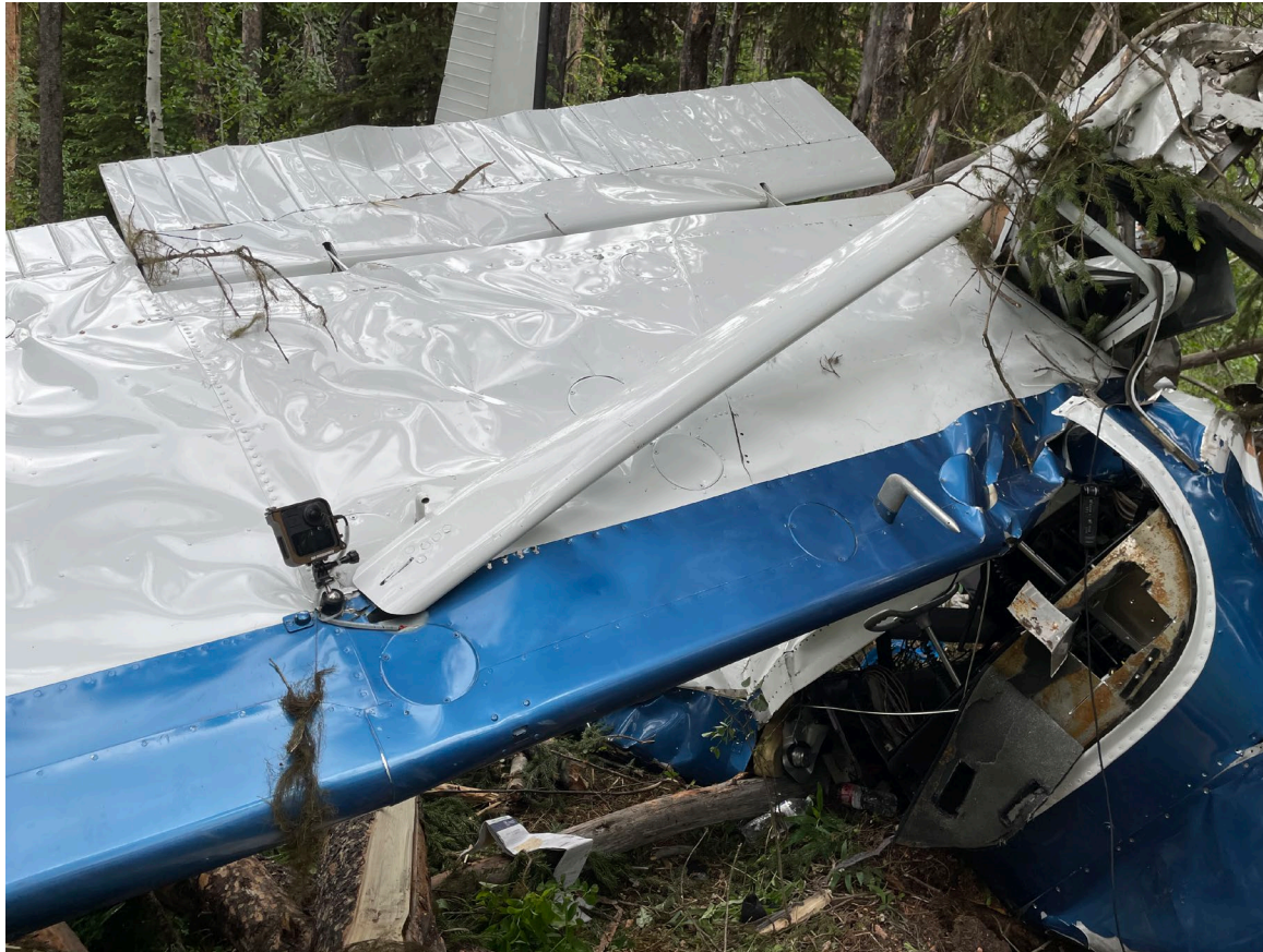
Photograph 4 - Video camera attached to the left wing.
