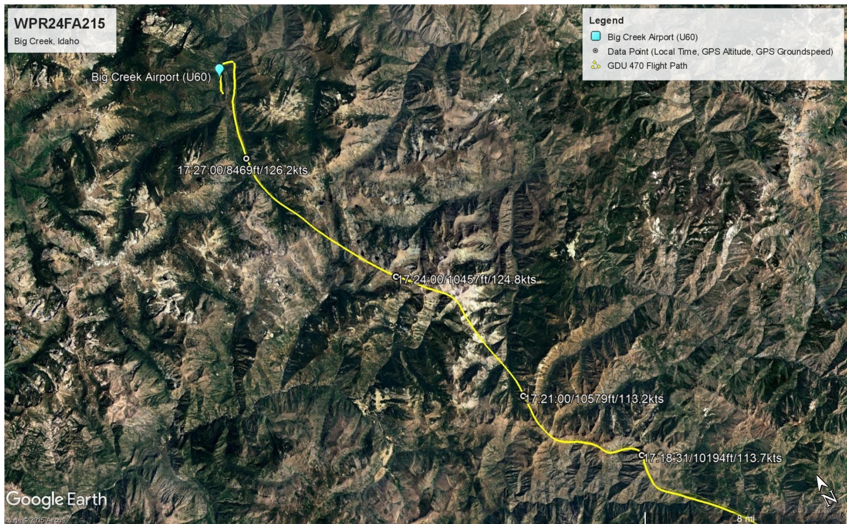
Figure 6. Google Earth overlay showing approximately the last 14 minutes of the accident flight recorded on the GDU 470.
