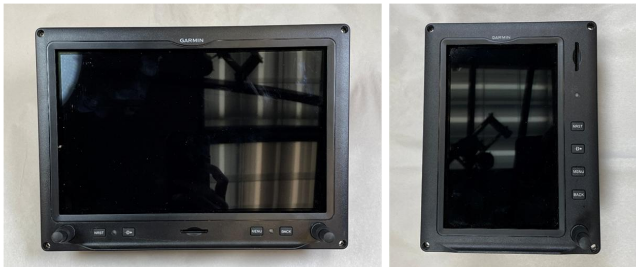
Figure 1. Photos of the front of GDU 460 (left) and GDU 470 (right), as received.
