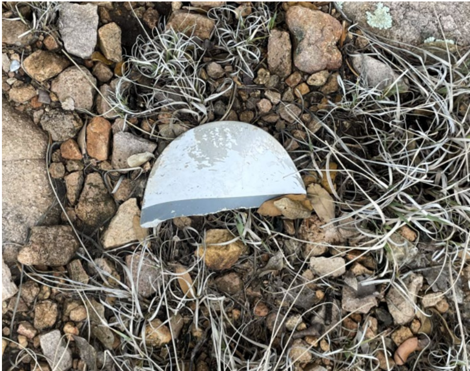
- Photo #2 -Tip fracture of another blade.
