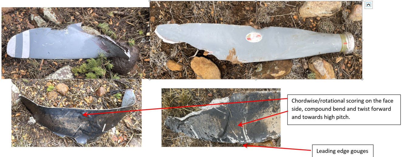
- Photo #1 - Montage of fractured blade
