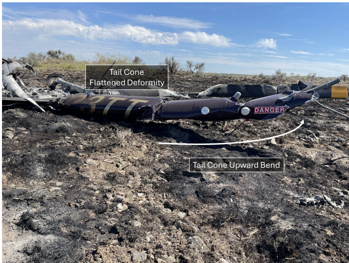
Figure 2. Tailcone. Fuselage end on the left, bear box end on the right.
