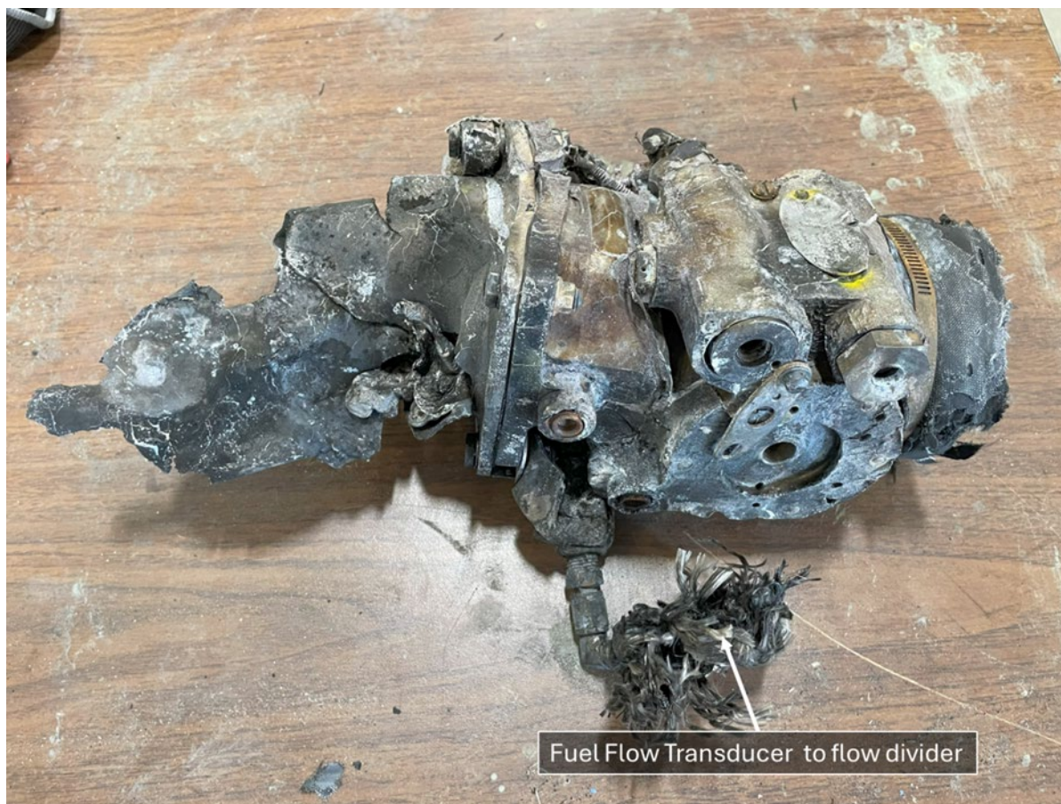
Figure 20. Line D, fractured end.
