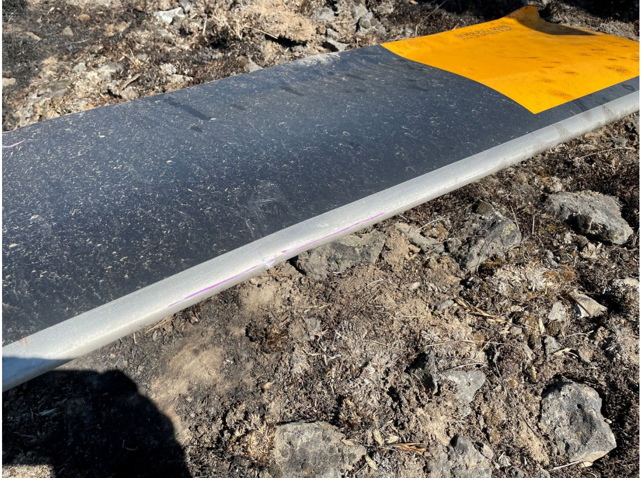
Figure 8. A section of Blade B showing color transfer like the color of the fuselage and tailcone paint.
