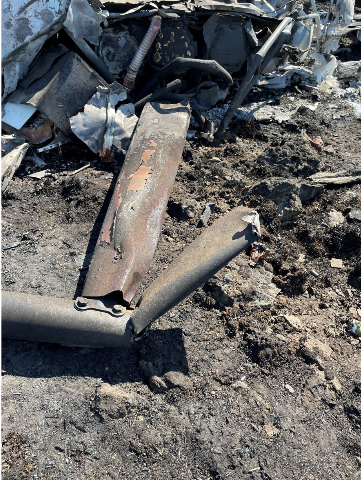
Figure 12. Left skid, aft end.
