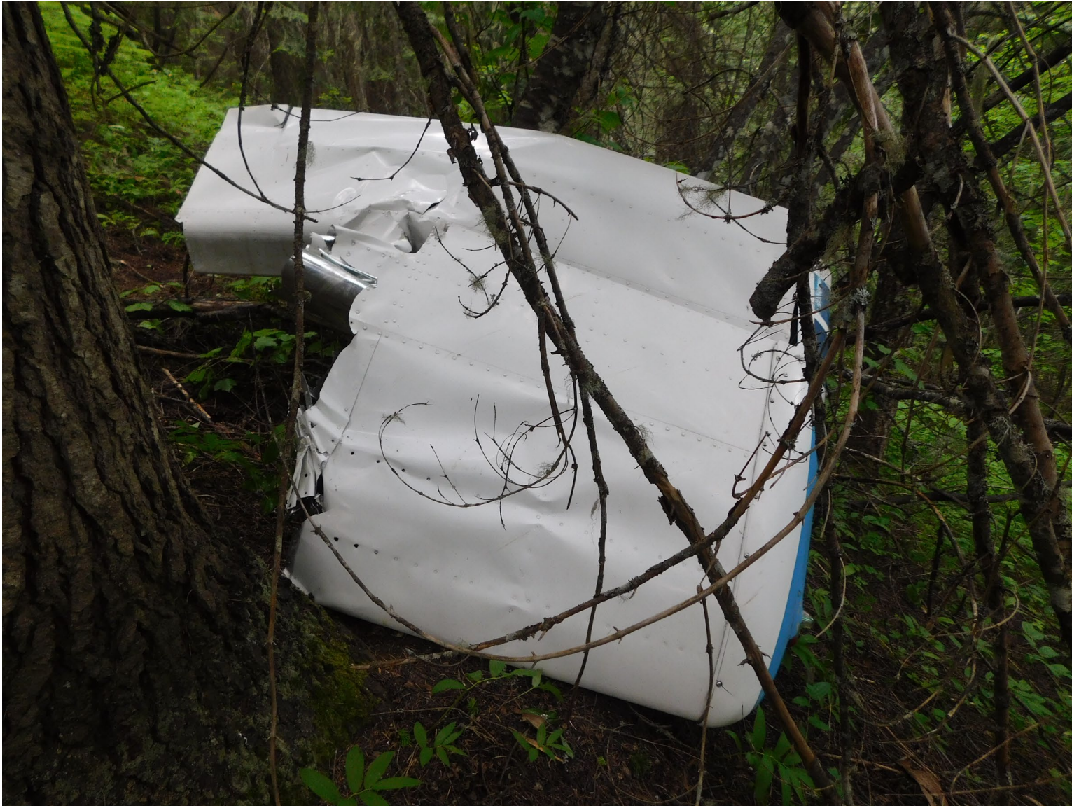
Photograph 5 - Outboard portion of left wing with aileron attached.
