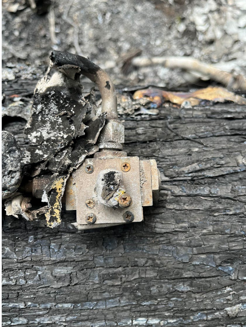
Figure 4. Fuel selector valve, as observed on fallen tree. (Courtesy of Textron)
