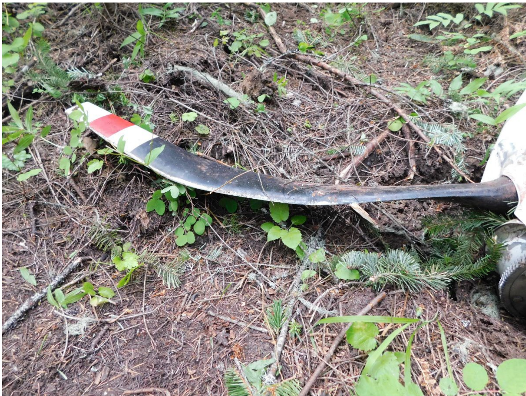
Figure 7. Forward bending of propeller blade.
