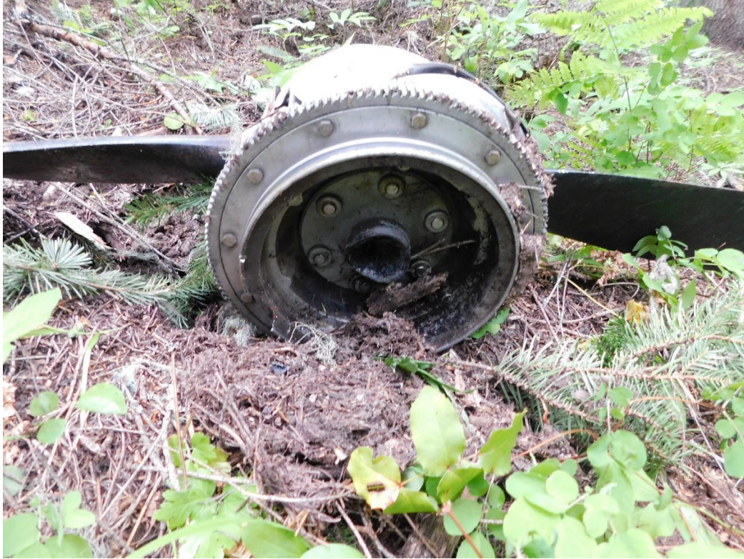
Figure 6. Propeller assembly at aft side of hub.
