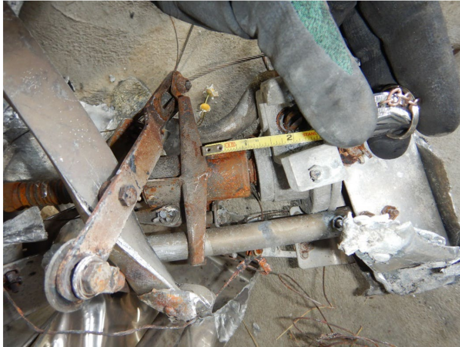
Figure 4. Measurement between the jackscrew motor and jackscrew carrier (Courtesy of Textron)
