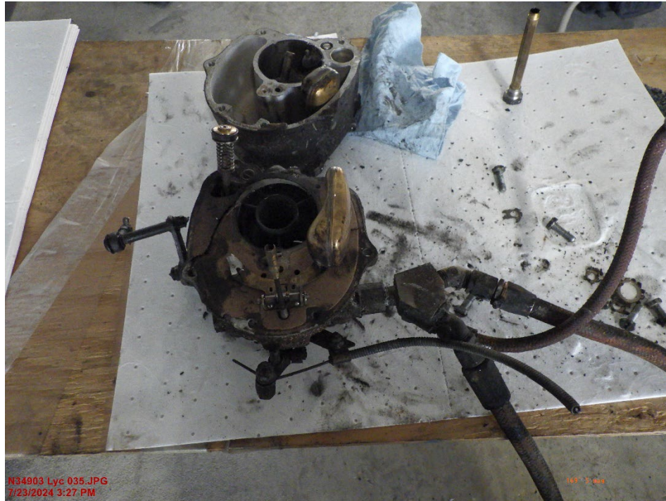
Figure 13. Disassembled carburetor (courtesy of Lycoming)
