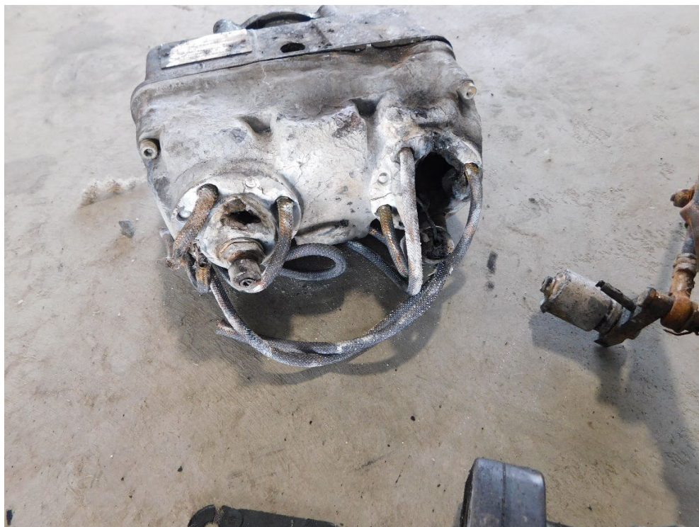
Figure 8. Single drive dual magneto after removal from engine.
