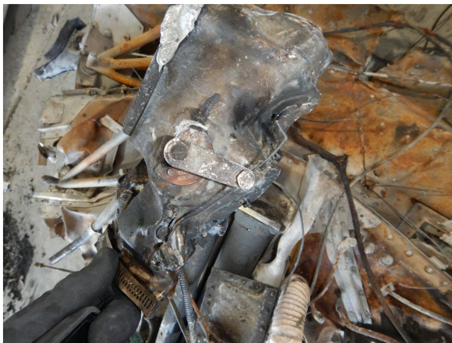
Figure 5. Carburetor heat control arm and airbox (Courtesy of Textron)
