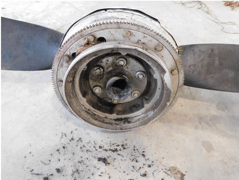
Figure 17. Aft view of propeller hub assembly and aft side of crankshaft flange.
