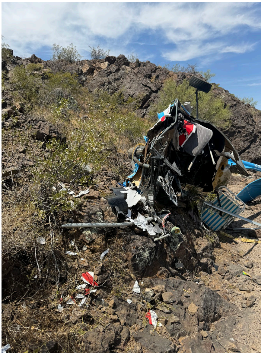
Photograph 5 - View of impact damage to the nose section of the airplane
