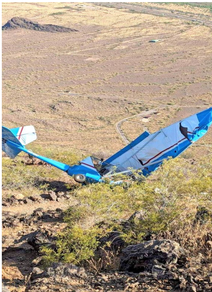
Photograph 1 - View of the accident airplane shortly after impact before first responder occupant extrication, showing damage to the right wing (Courtesy of social media)
