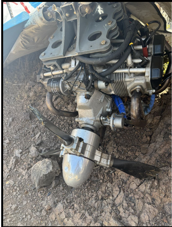
Figure 5: View of the inverted engine with unremarkable propeller hub extension, hub, damaged propeller blade and minor damage sustained to the spinner.
