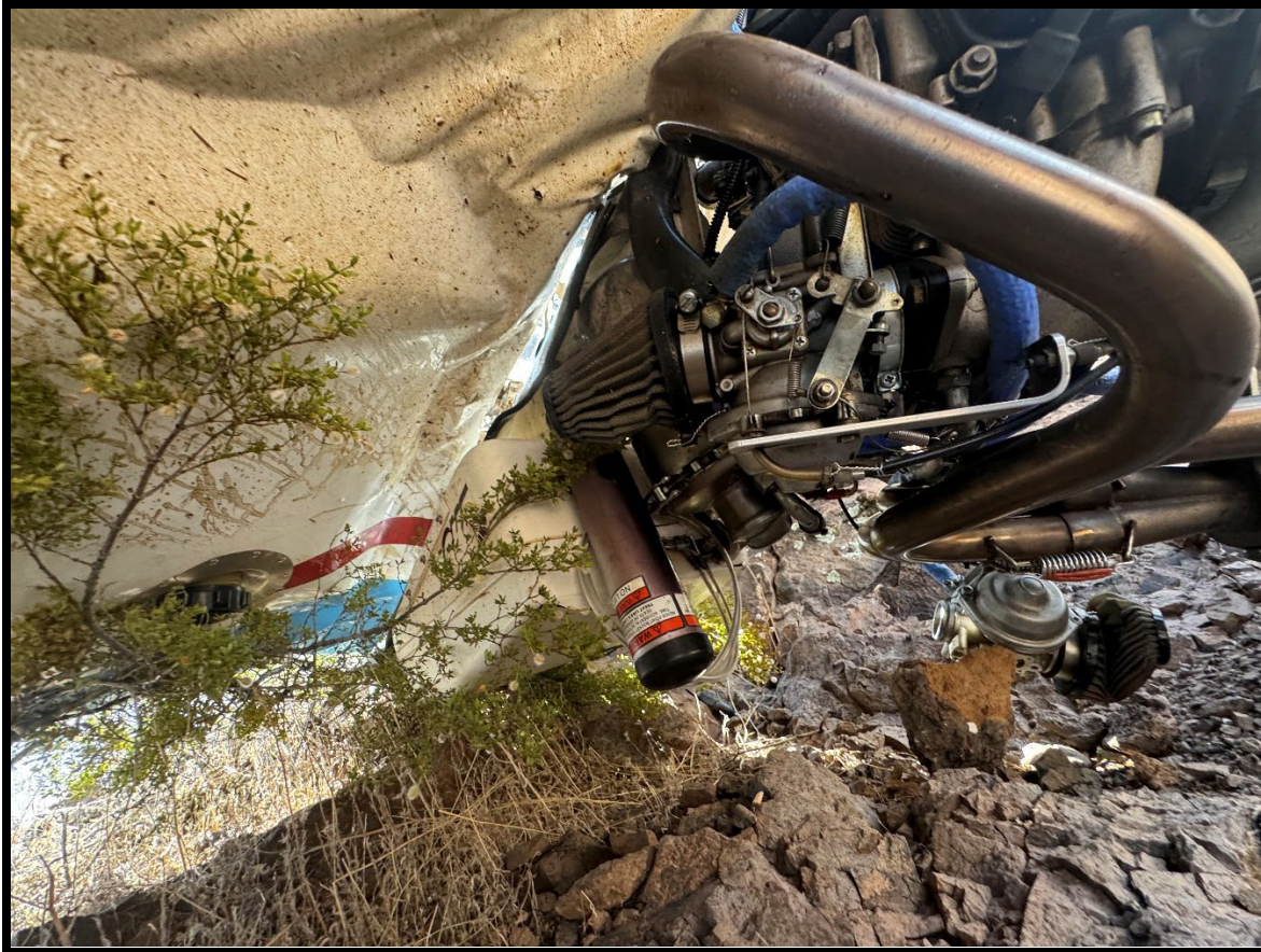
Figure 3: View of the inverted engine and damage to the 1/3 carburetor.
