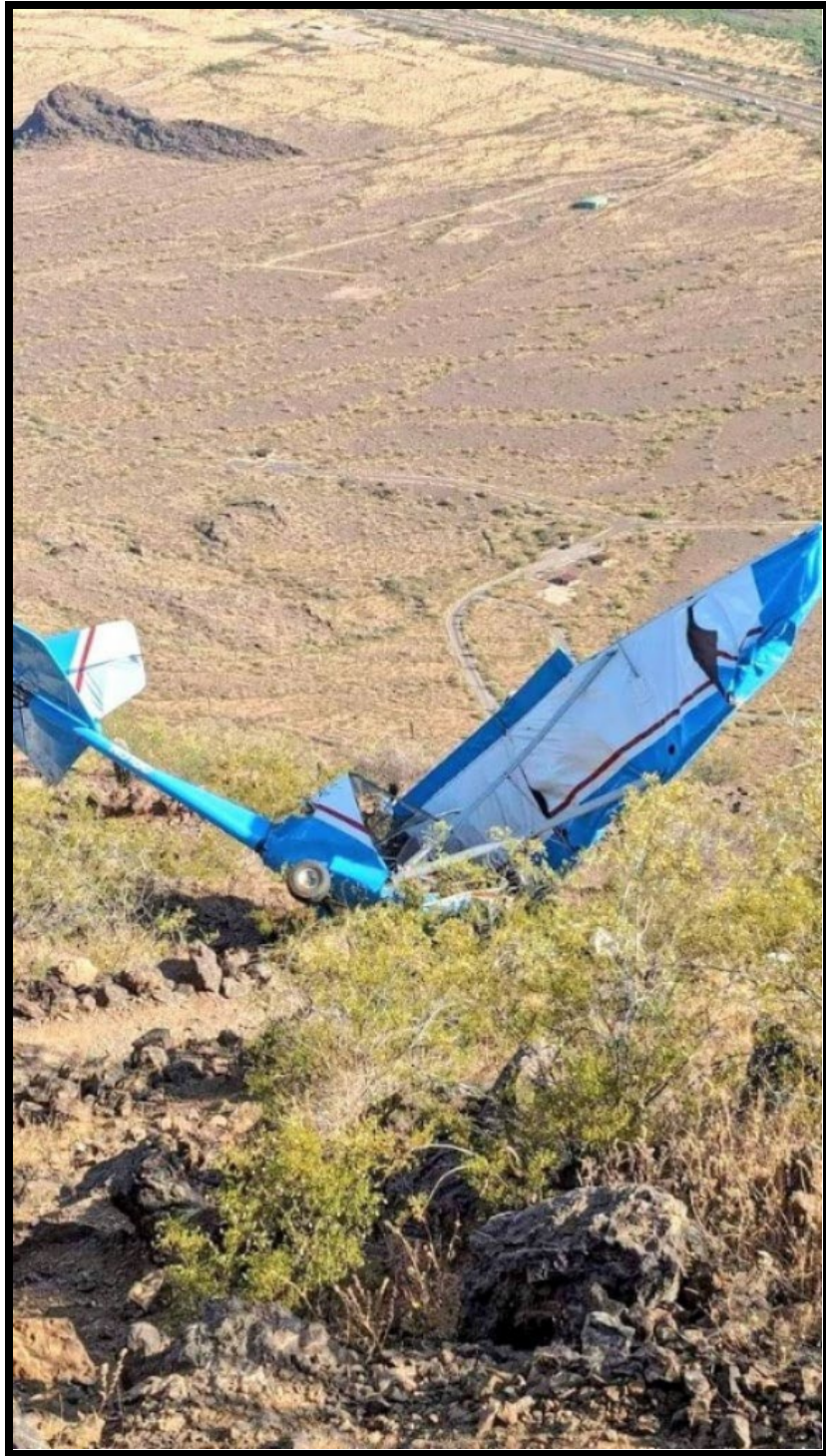
Figure 1: View of the airplane in the initial impact position, prior to first responder aircraft manipulation to facilitate extrication (Courtesy of social media).
