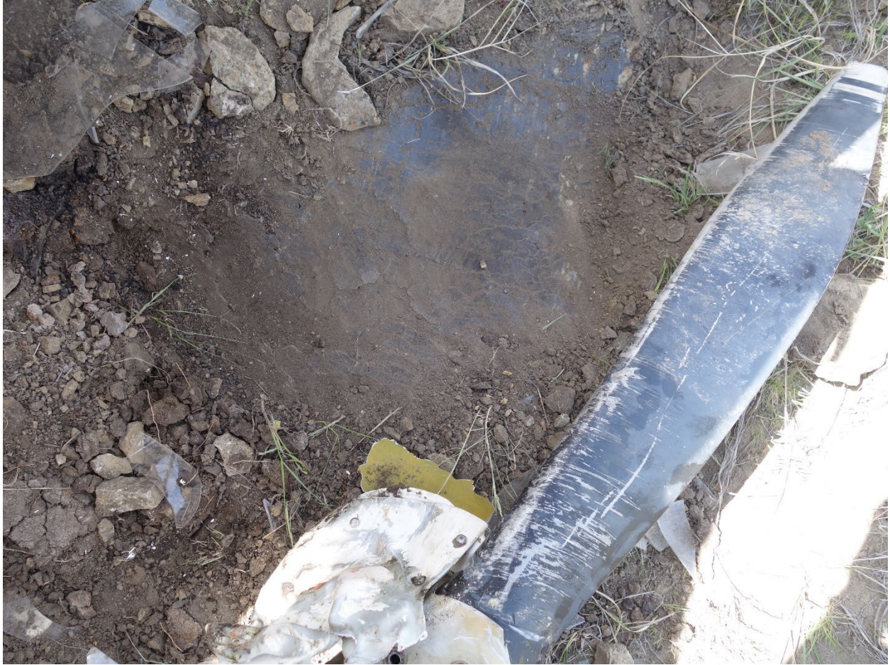
Figure 3. Image showing the first point of probable impact. The propeller is positioned for scale.
