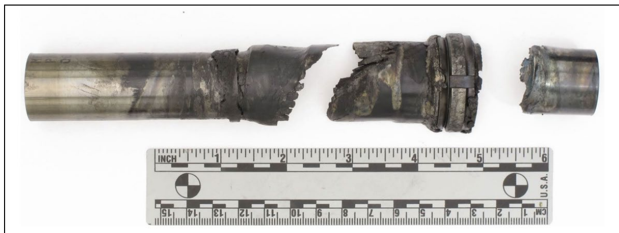
Photograph 4 - Fractured Turbine to Compressor Coupling Shaft
