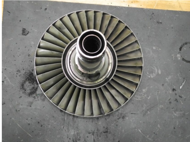
Photo 27 - 4 th Stage Turbine Wheel - Intact
