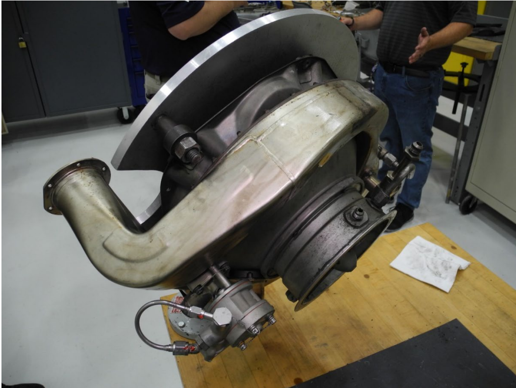
Photo 9 - Compressor Module - Undamaged
