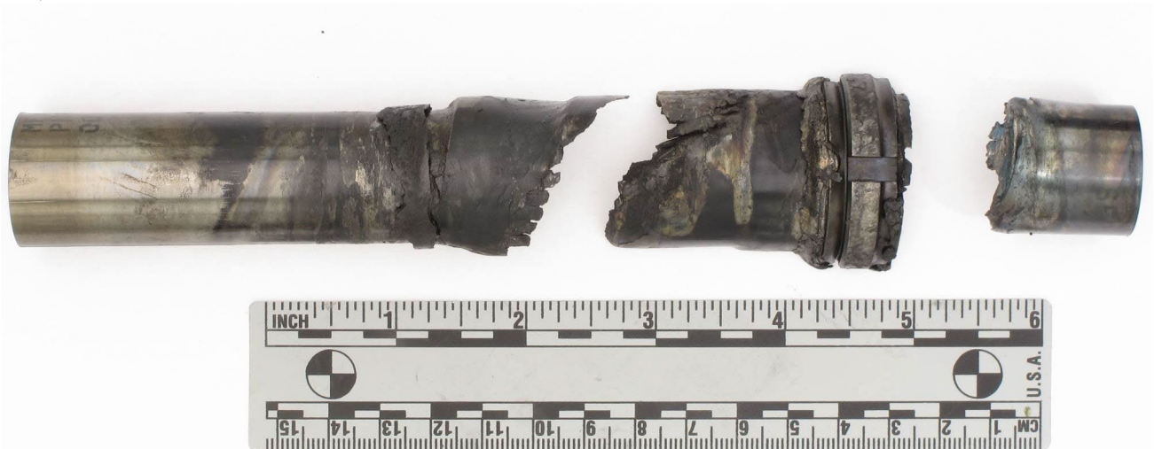
Photo 30 - Turbine-to-Compressor Coupling Shaft - Fractured - Courtesy RR
