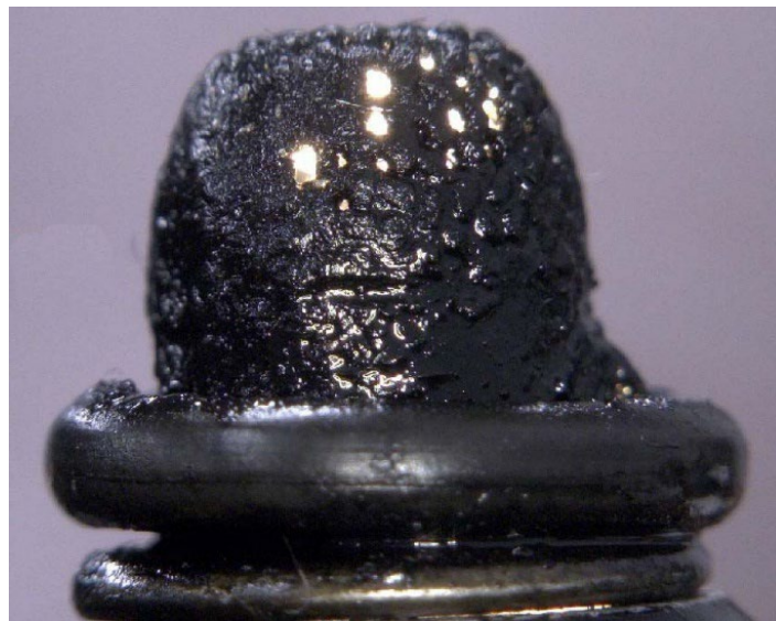
Photo 22 - Piccolo Tube Oil Screen - Courtesy RR
