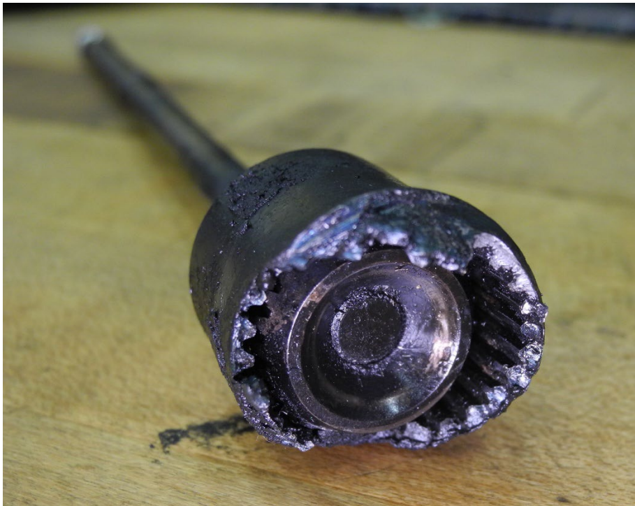
Photo 32 - Turbine-to-Compressor Coupling Shaft Was Deformed Over Tie Bolt Nut
