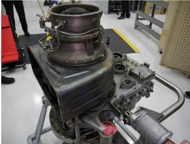
Photo 23 - Exhaust Collector Support Housing - Intact
