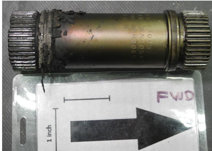
Photo 25 - PT-To-Pinion Gear Coupling - Note Thermal Distress
