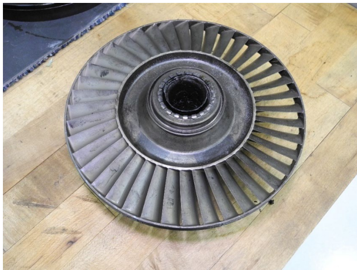
Photo 28 - 3 rd Stage Turbine Wheel
