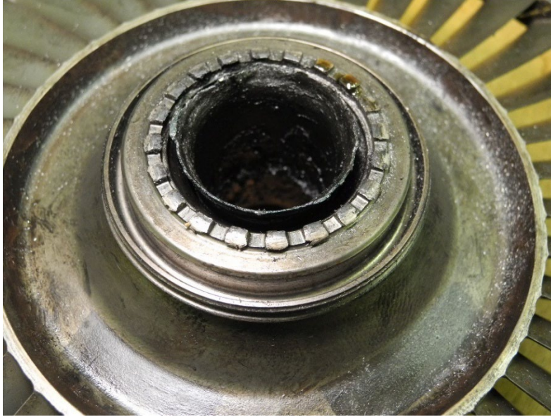
Photo 29 - 3 rd Stage Turbine Wheel Curvic Coupling - Rotationally Smeared
