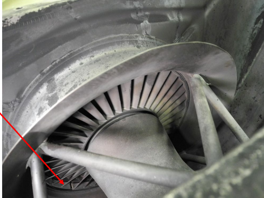
Photo 8 - 4 th Stage Turbine Wheel
