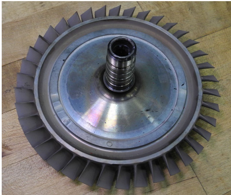
Photo 33 - 1 st Stage Turbine Wheel - Undamaged
