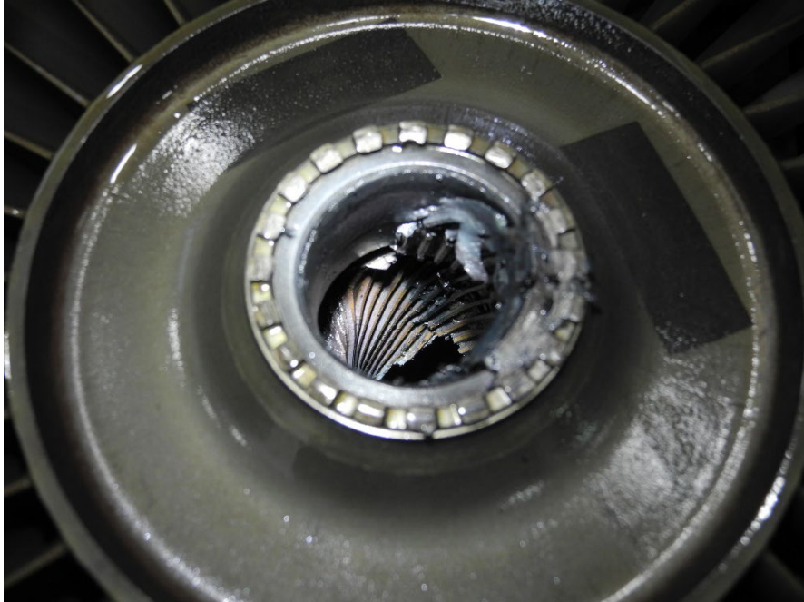
Photo 31 - 4 th Stage Wheel with Portion of the Deformed and Seized Turbine-to-Compressor Coupling Shaft
