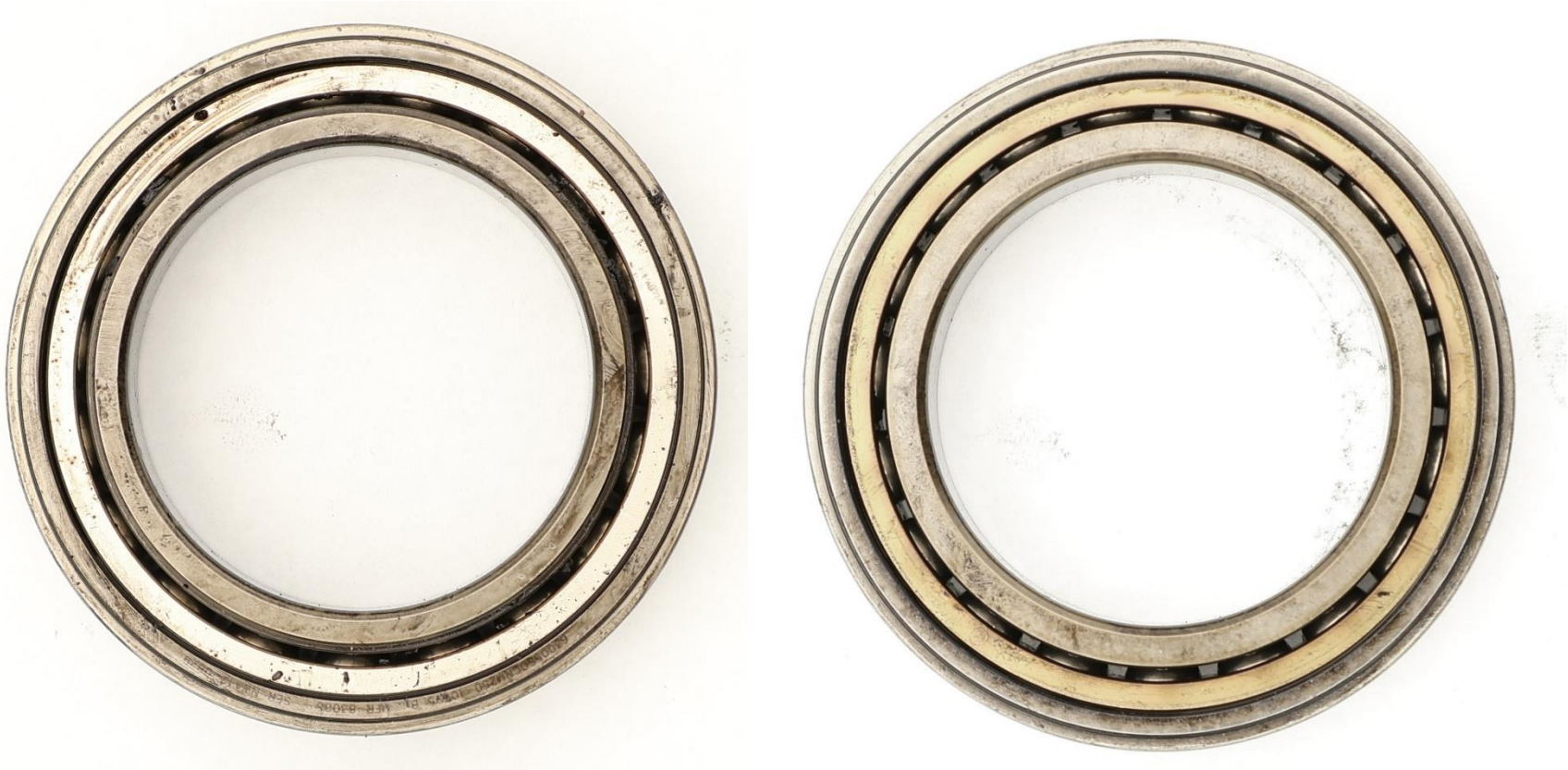
Figure 46. Overall forward looking aft (left) and aft looking forward (right) views of the No. 5 bearing in the as-received condition.
