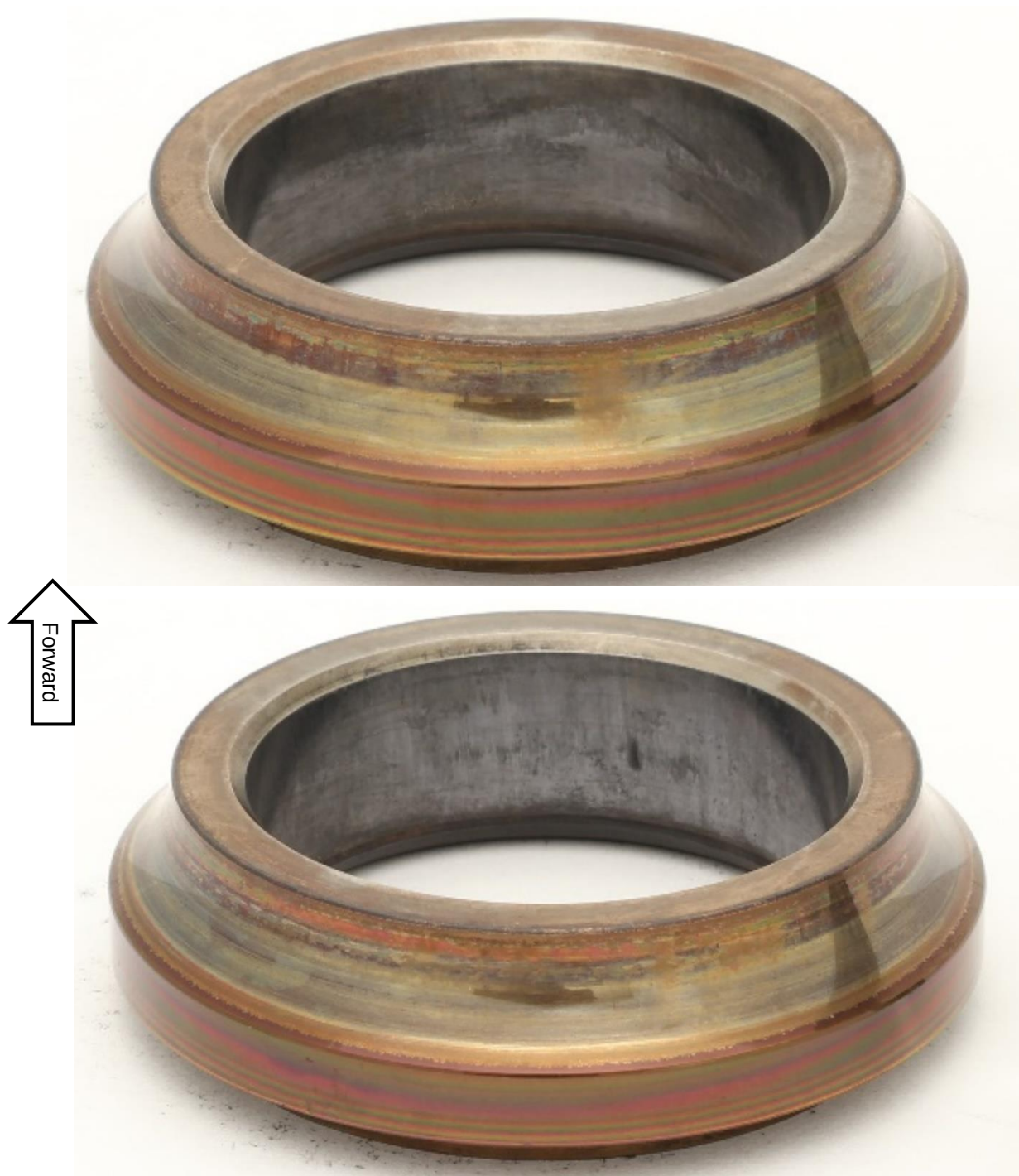
Figure 42. Detailed views of the No. 2 bearing aft inner race. Each image is rotated approximately 180° from the previous.
