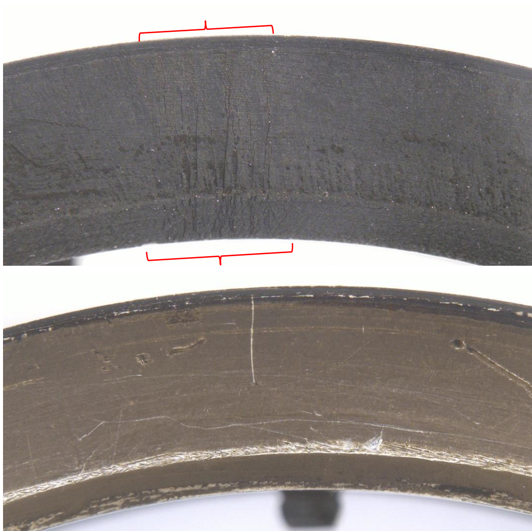
Figure 39. Detailed views of the No. 2 bearing separator forward (top) and aft (bottom) rail. The forward rail exhibited a dark discoloration and linear features (red braces).
