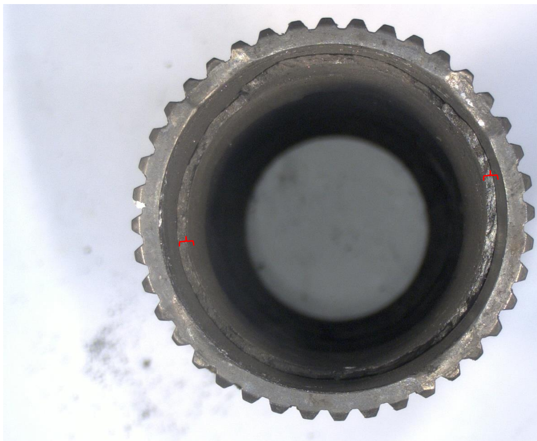
Figure 33. Overall aft looking forward view of the pinion gear coupling showing turbine to compressor coupling material (red braces) in the inner diameter.
