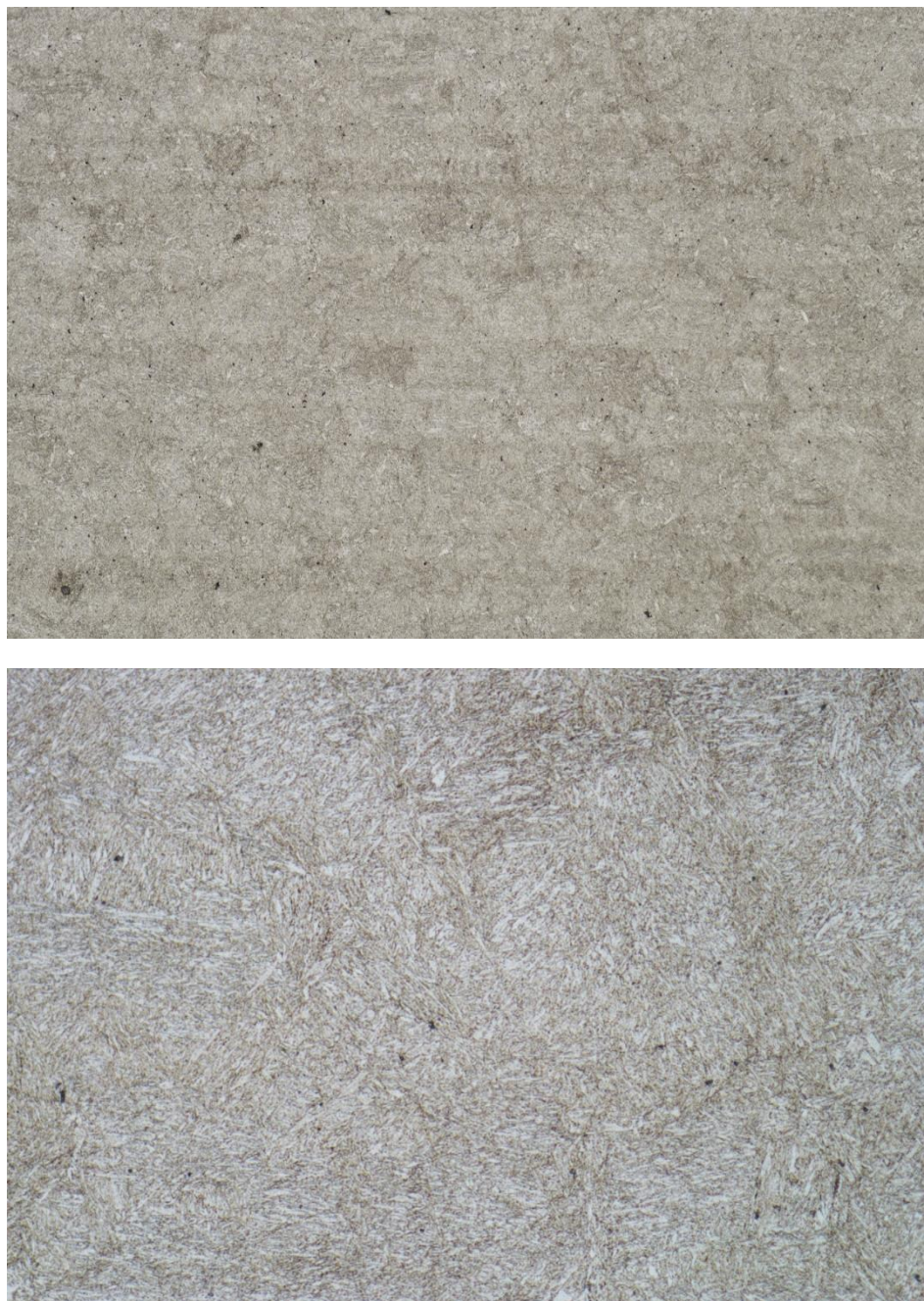
Figure 24. Representative microstructure of the PT inner shaft core material from cross-section P3 (see Figure 21). Etchant: Nital.
