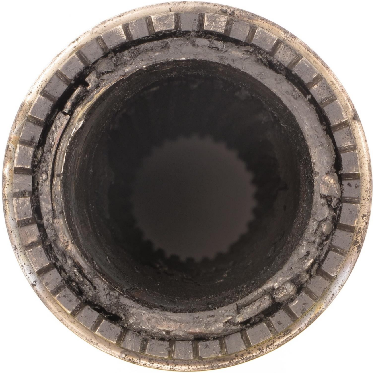
Figure 4. Overall aft looking forward views of the power turbine outer shaft in the as-received condition. Smeared PT inner shaft, PT inner coupling nut, and turbine to compressor coupling material was observed on the aft end along with coked oil.
