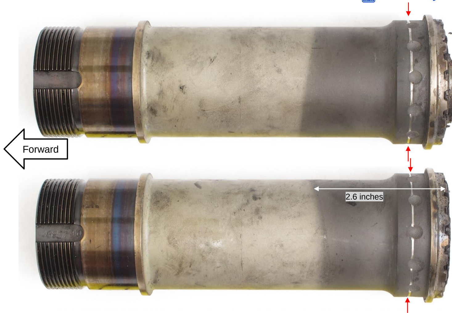
Figure 3. Overall outboard looking inboard views of the power turbine outer shaft in the as-received condition. Each image is rotated approximately 180° from the previous. The red arrows indicate circumferential score marks consistent with disassembly damage from the PT coupling nut.
