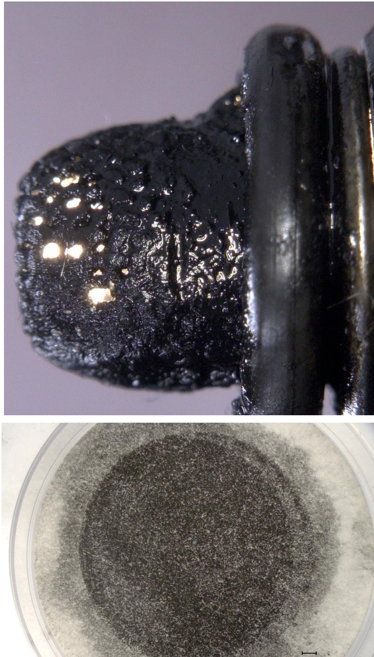
Figure 30. Top: Detailed view of the oil screen back lit from the aft end. Dark deposits consistent with coked oil product were observed around a majority of the screen surface. Bottom: overall view of filtered product from the oil screen. The product consisted of a black powder type material consistent with coked oil.
