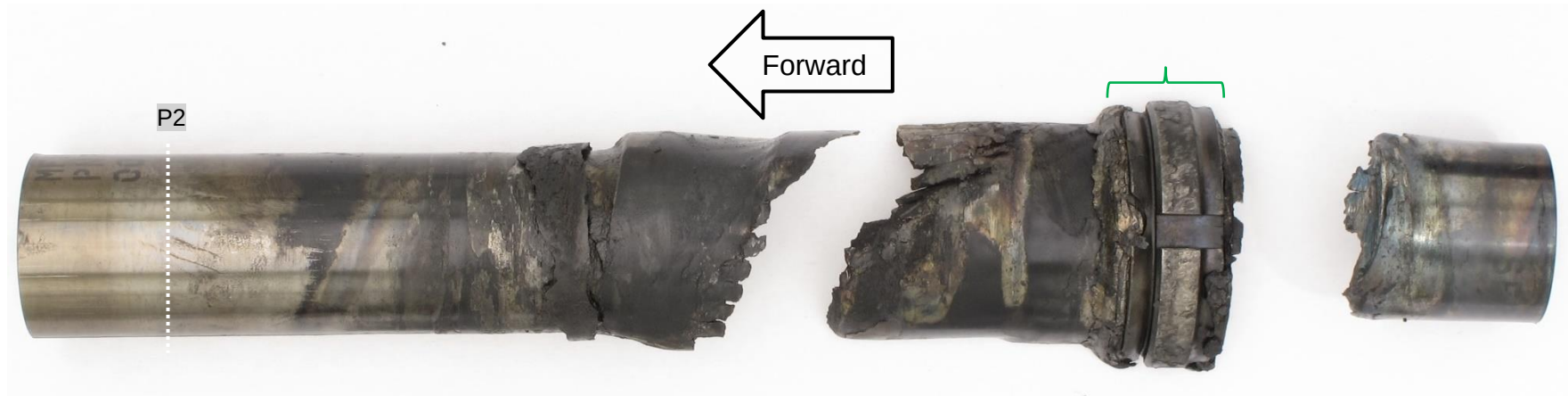
Figure 9. Overall view of the turbine to compressor coupling pieces. Not pictured: portions of the turbine to compressor coupling embedded in the 4 th stage turbine wheel (see Figure 6) and the PT outer shaft (see Figure 5). The green brace indicates PT inner shaft material and the PT inner coupling nut adhered to the turbine to compressor coupling. The white dashed line indicates the approximate cross-section (P2) selected for metallographic examination as shown in Figure 17.
