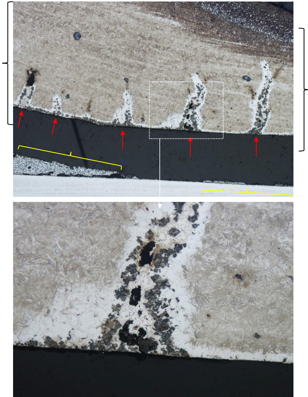
Figure 13. Detailed metallographic images of the turbine to compressor coupling (black braces) and PT inner shaft material (yellow braces) (location C from Figure 10) showing localized areas of transformed material (red arrows). Melted PT inner shaft material is indicated by the yellow braces. Etchant: Nital.
