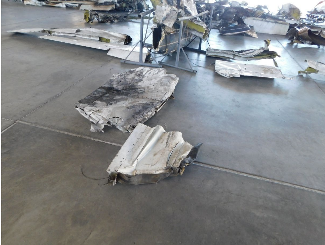
Figure 6. Rudder and upper section of vertical stabilizer
