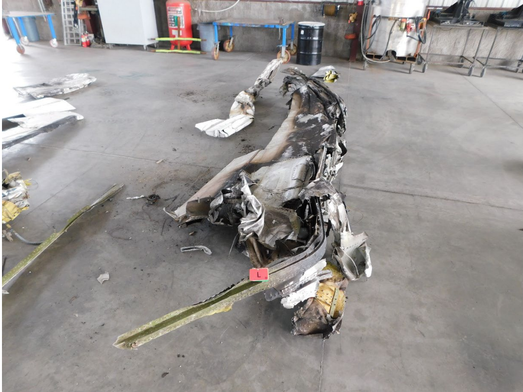
Figure 2. Left wing, aileron, outboard flap
