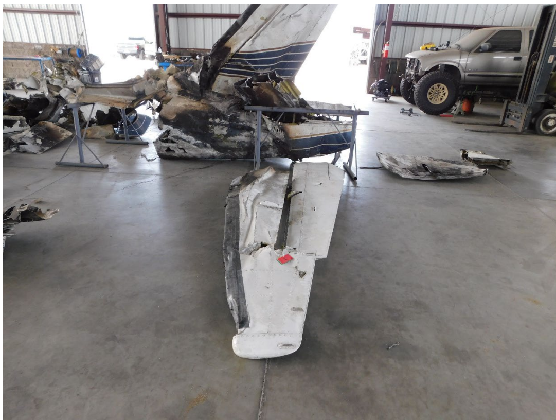
Figure 4. Left horizontal stabilizer and elevator
