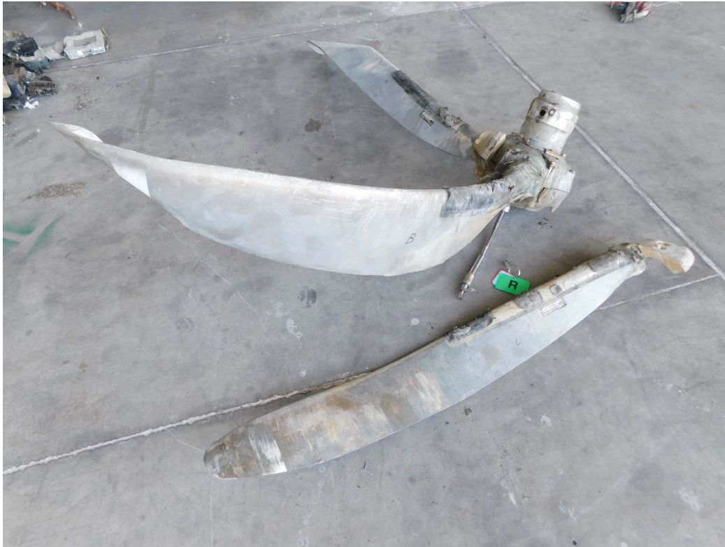
Figure 12. Right propeller assembly
