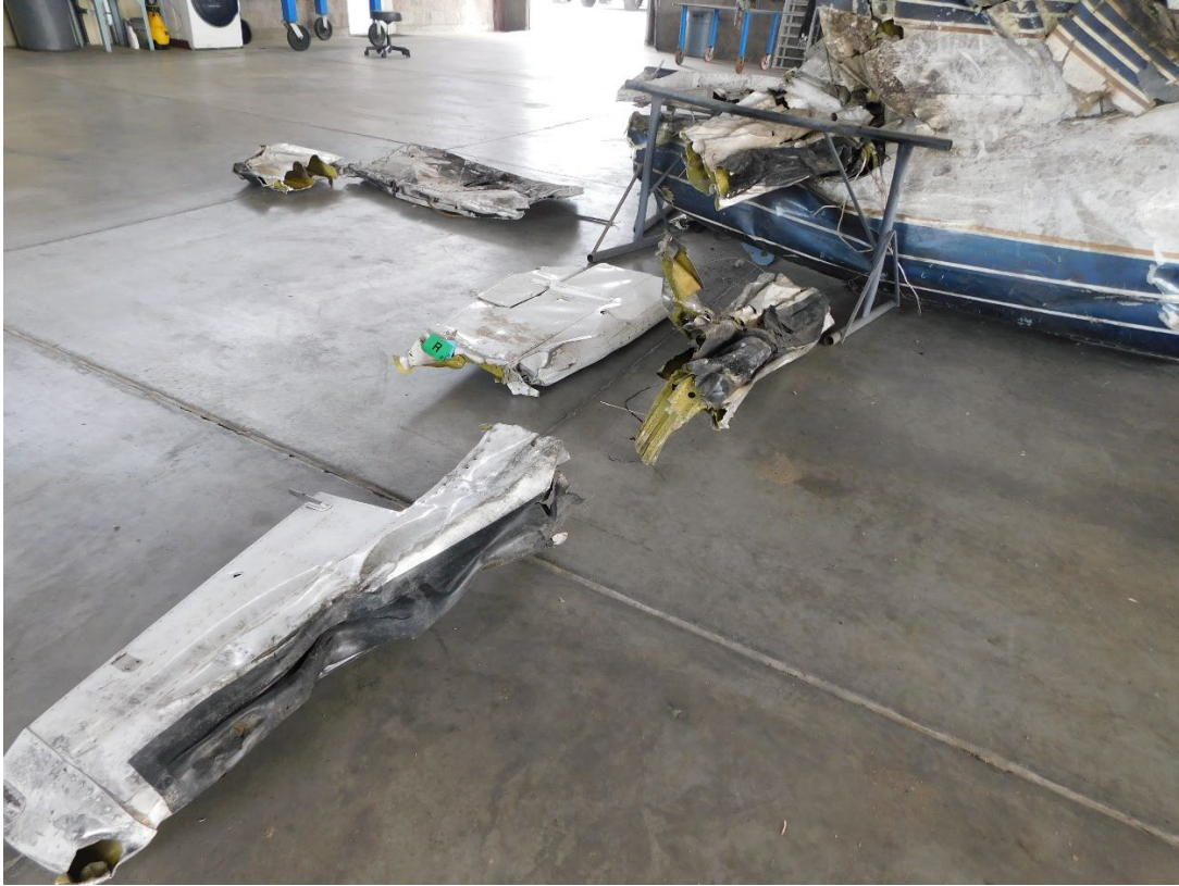
Figure 5. Right horizontal stabilizer and elevator
