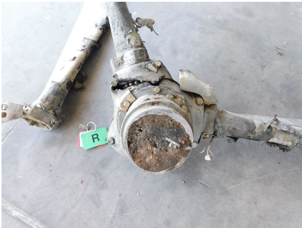
Figure 8. Wiring observed present with two propeller blade de-ice boots
