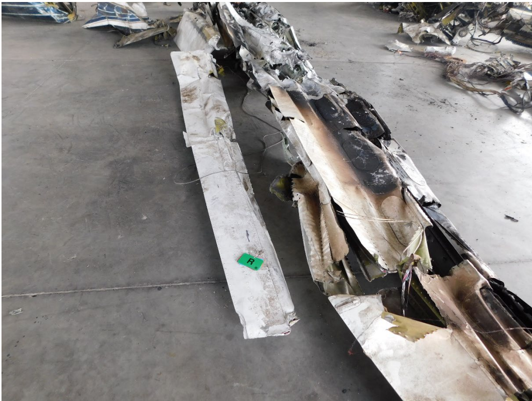
Figure 3. Right wing, aileron, outboard flap
