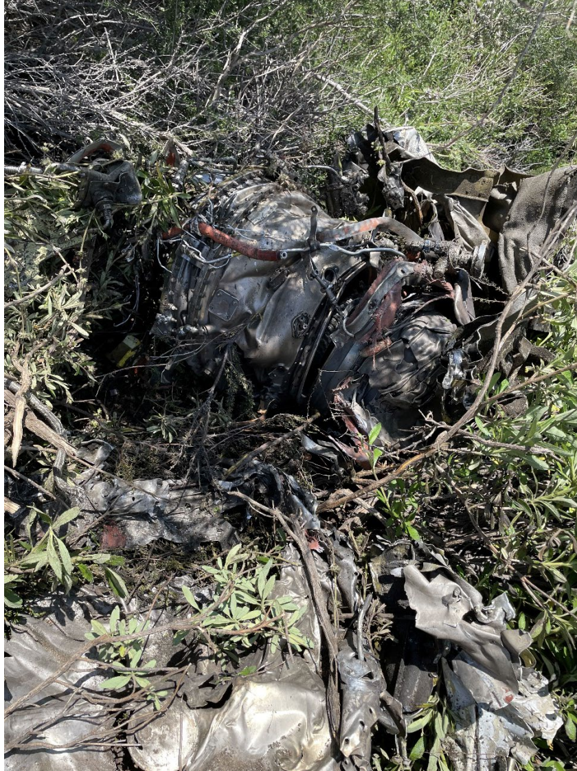
Figure 6. Engine power section located on north slope
