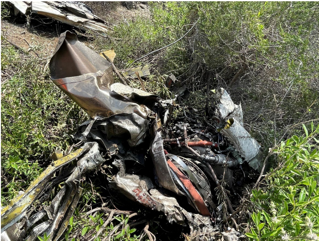
Figure 5. Engine power section located on south slope
