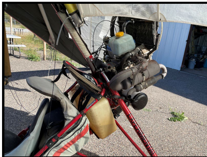
Figure 5: Fuel in the fuel cell is greater than 1/3 full
