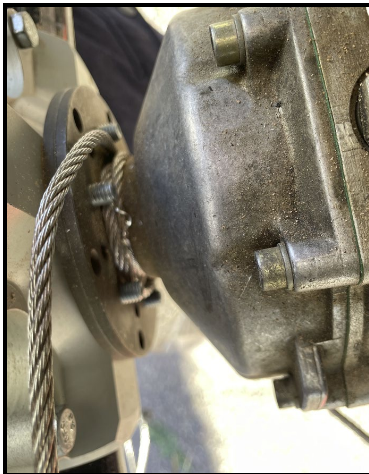
Figure 2: View of right side, rear flying wire wrapped twice around propeller flange
