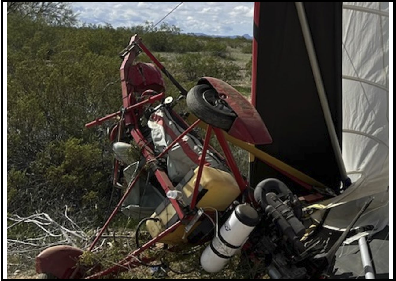
Figure 1: View from aft to forward, of the carriage keel left bending impact signature
