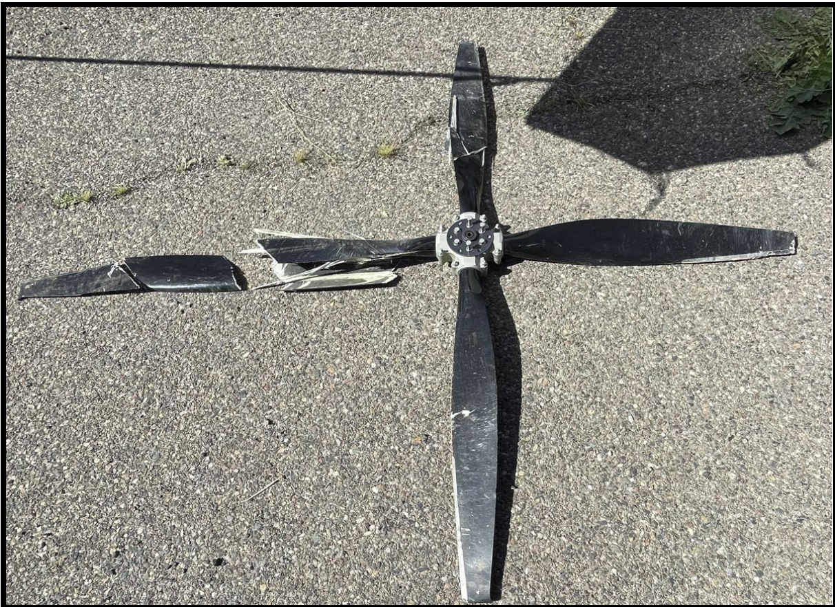
Figure 6: View of damage to the propeller blades
