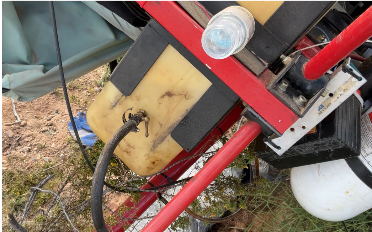
Photograph 3 - View of fuel selector in the open position (Courtesy of LEA)
