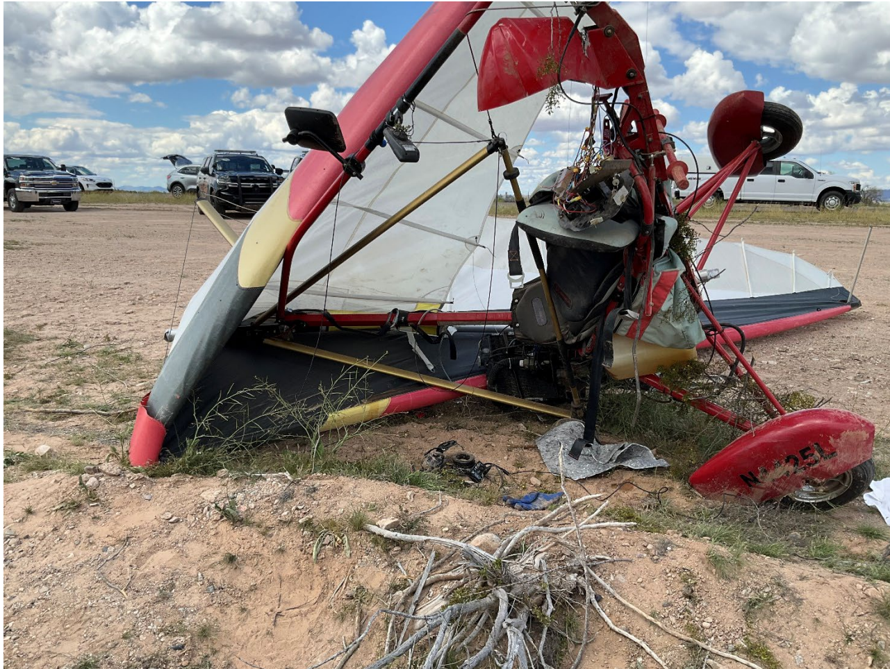
Photograph 1 - Forward to aft view of aircraft with mesquite tree attached to lower carriage (Courtesy of LEA)
