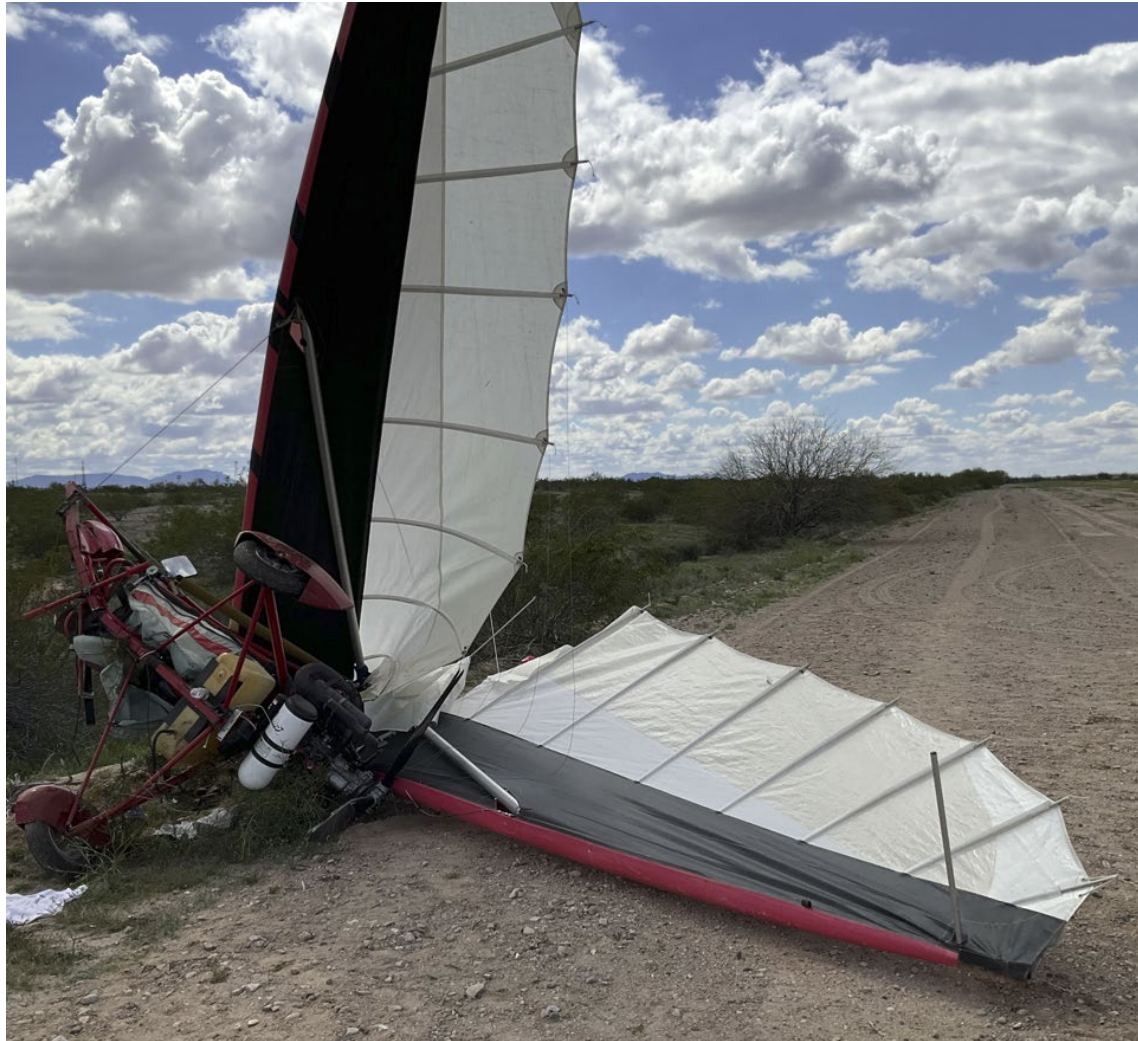
Photograph 2 - Bottom view of inverted aircraft with damage to inboard sail and carriage keel (Courtesy of FAA)
