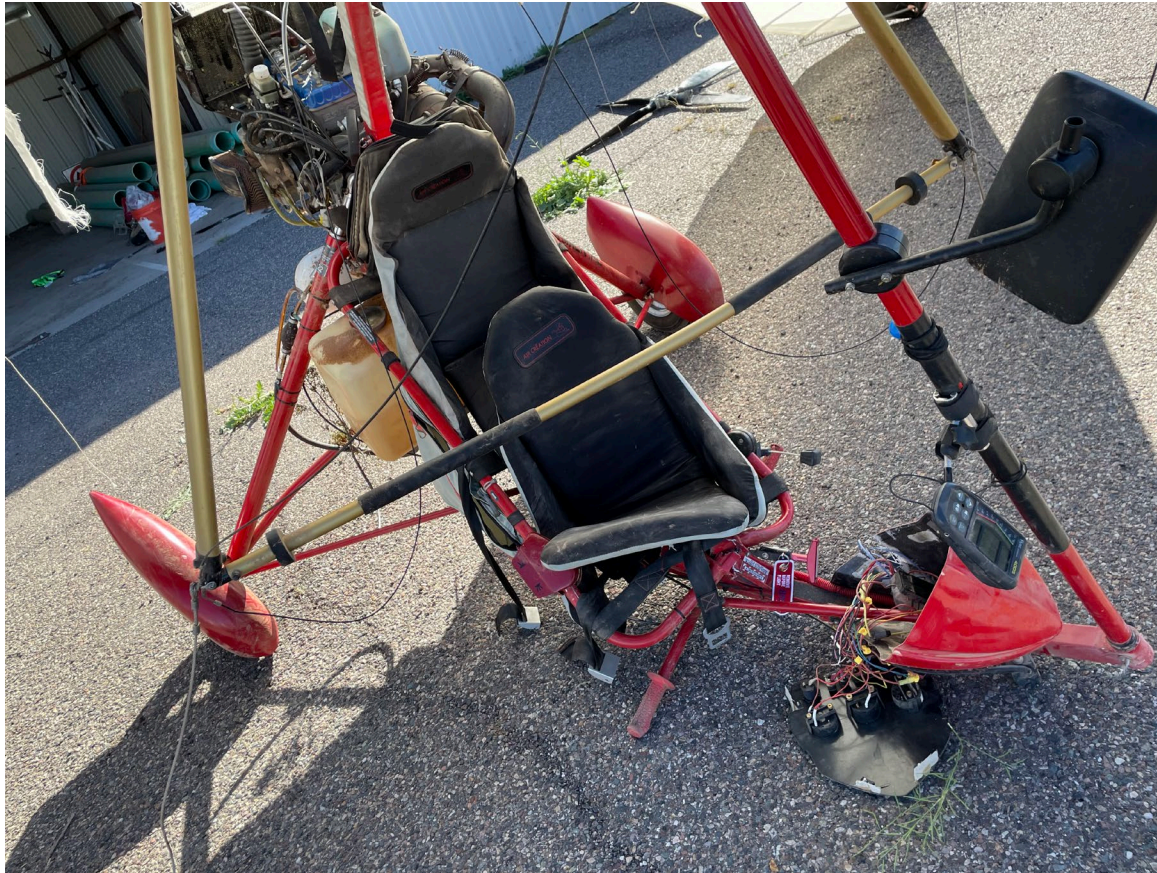
Photograph 4 - Front to aft view of the impact damage to carriage keel forward seat frame
