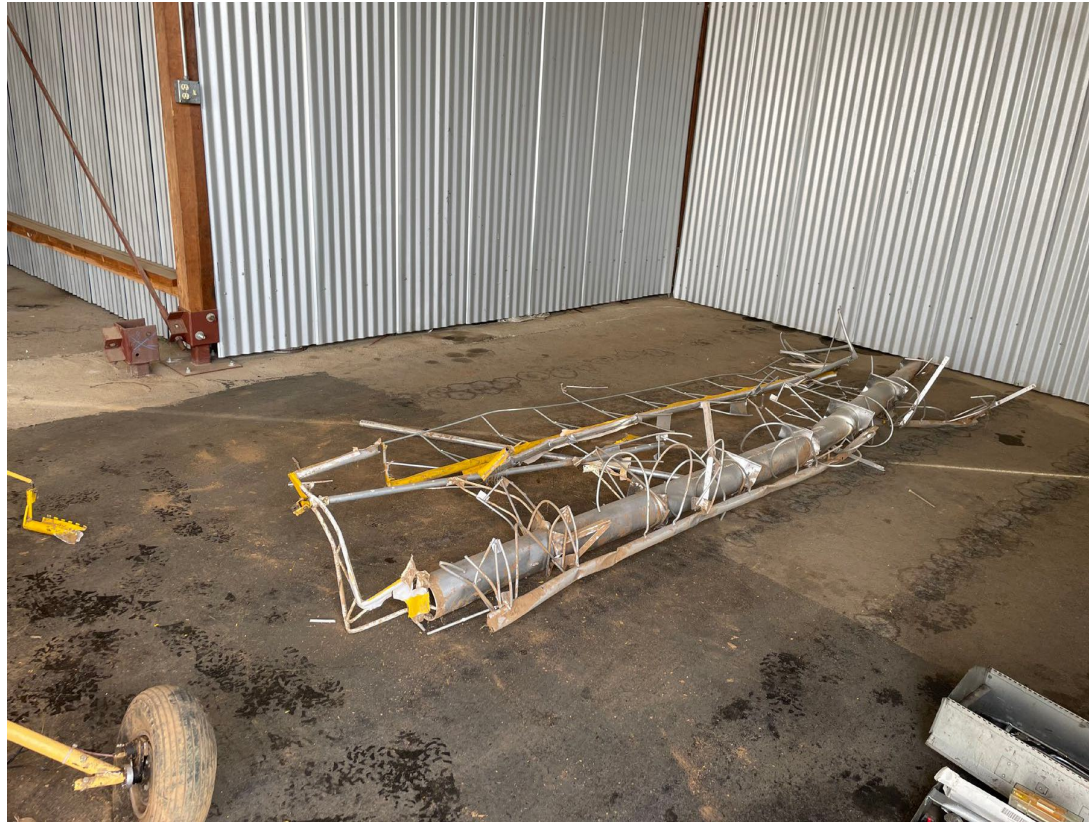
Photograph 6 - View of left-wing during examination
