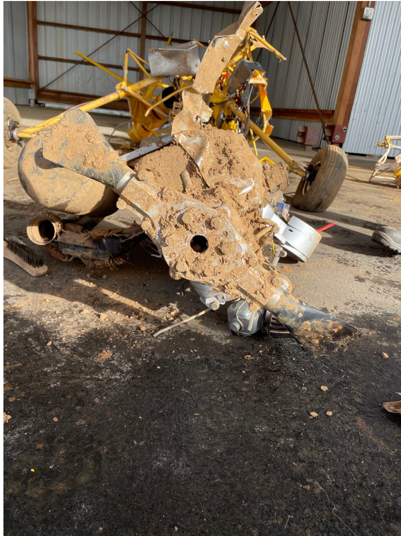
Photograph 4 - View of damaged propeller assembly
