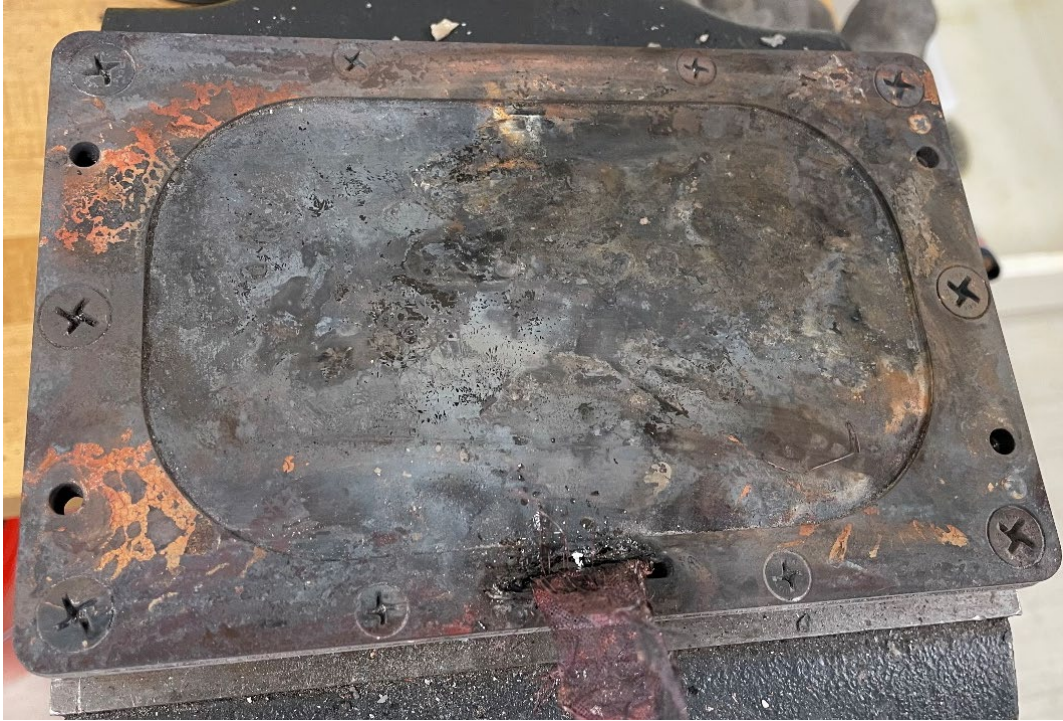
Figure 1. Heat damaged crash case of the CVR (view of bottom).
