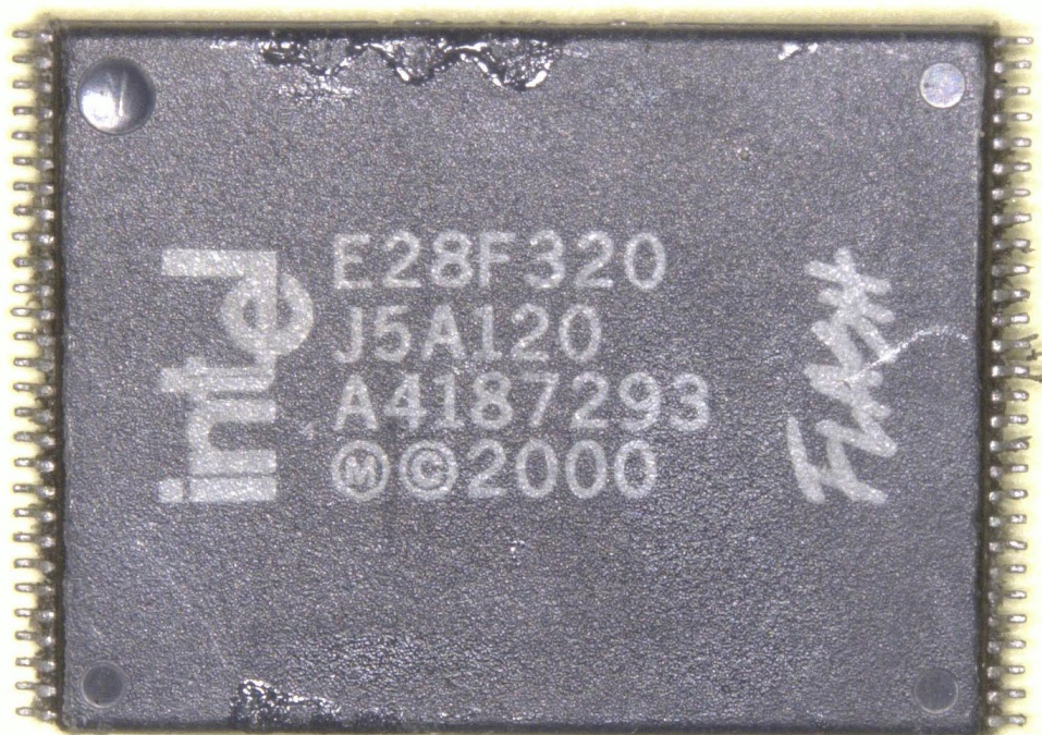
Figure 11. FLASH memory device after removal from the PCB (top view).
