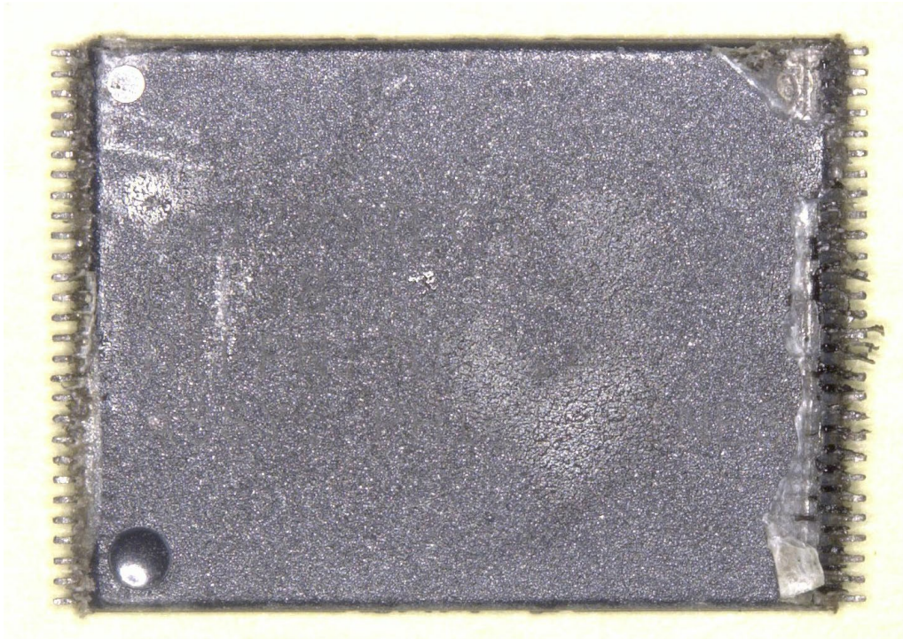
Figure 12. FLASH memory device after removal from the PCB (bottom view).
