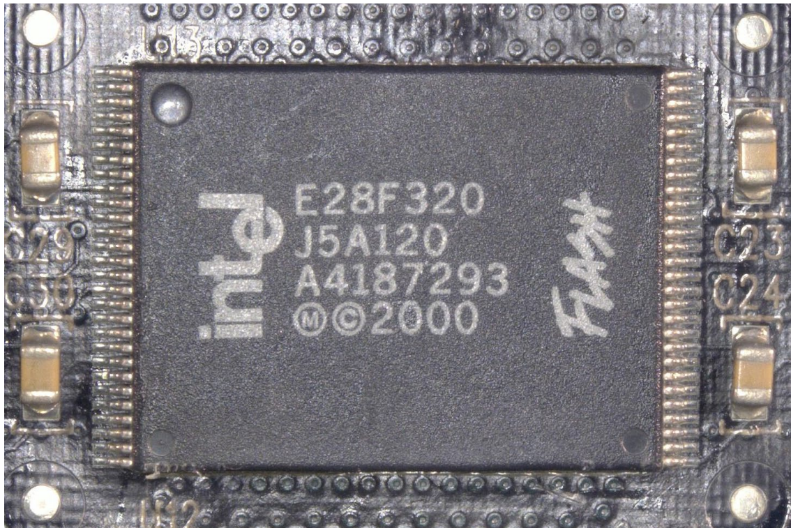
Figure 8. FLASH memory device mounted on accident memory module PCB before Parylene removal.
