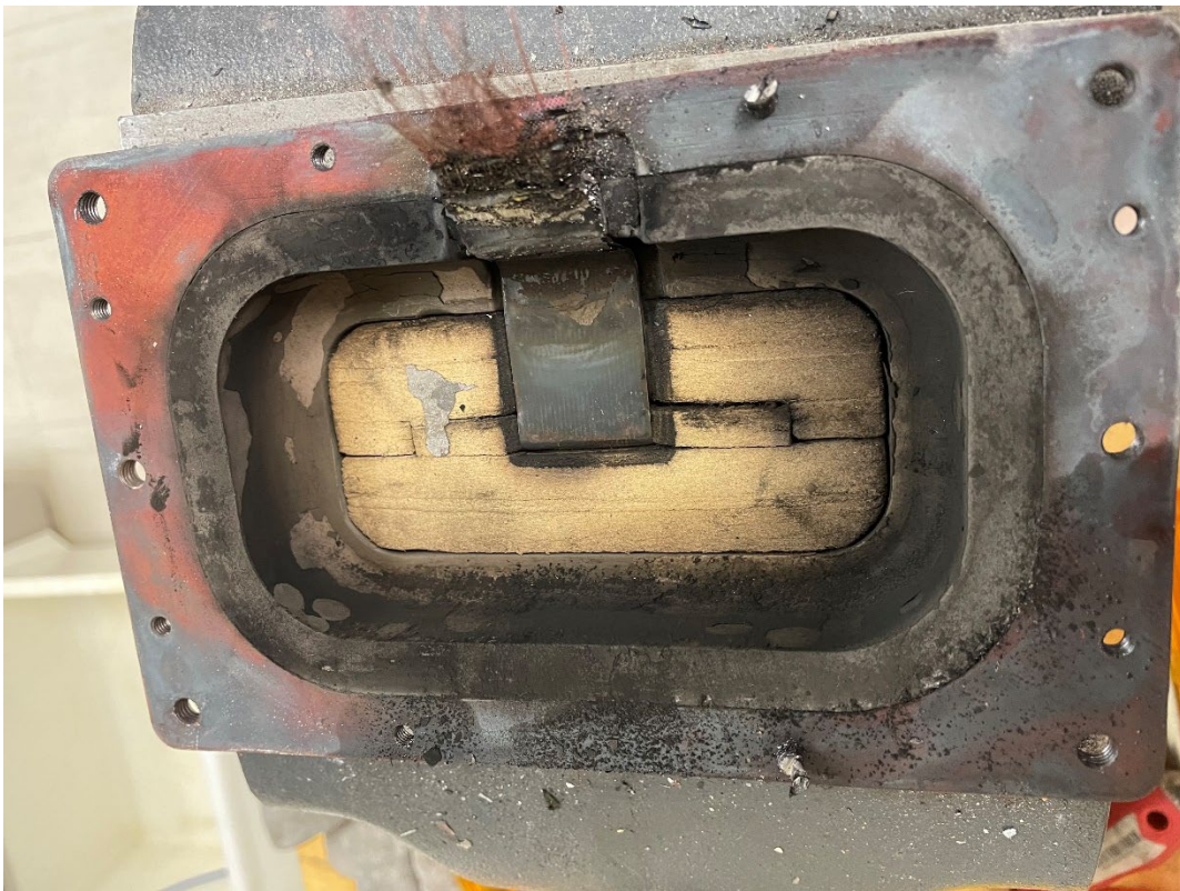
Figure 2. View of crash case opened to reveal heat insulation material and ribbon cable.
