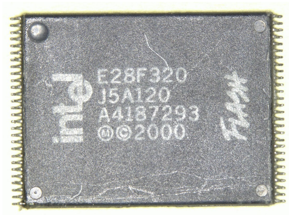
Figure 17. Top view of FLASH memory device after cleaning.
