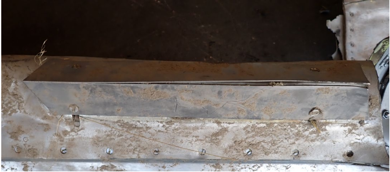
Figure 3: Stall spoiler (stall strip) at right wing leading edge
