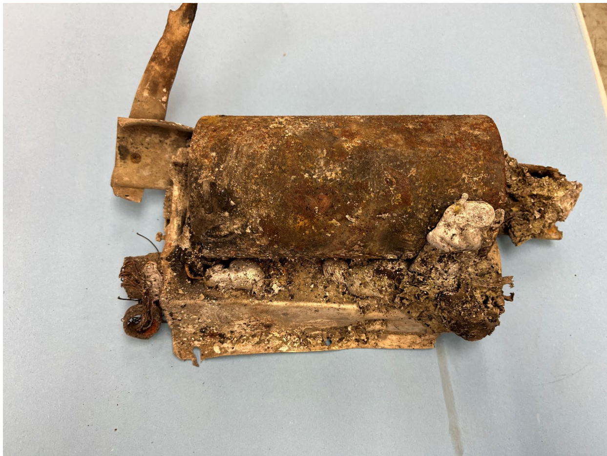
Figure 1. Damaged exterior of flight data recorder.
