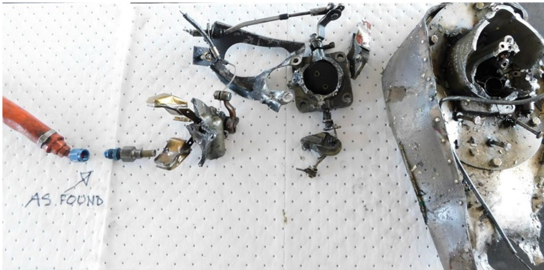
Figure 4: Output fuel line B-nut as found.
