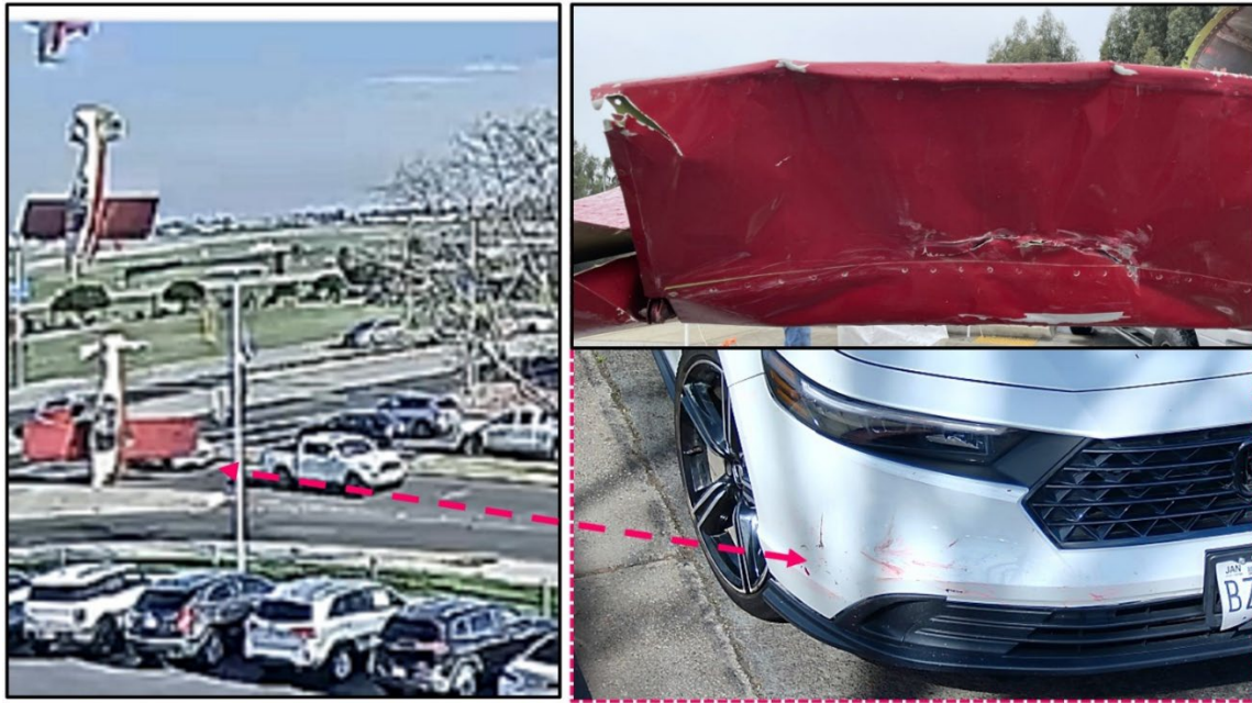
Figure 7: Left aileron vehicle impact damage
