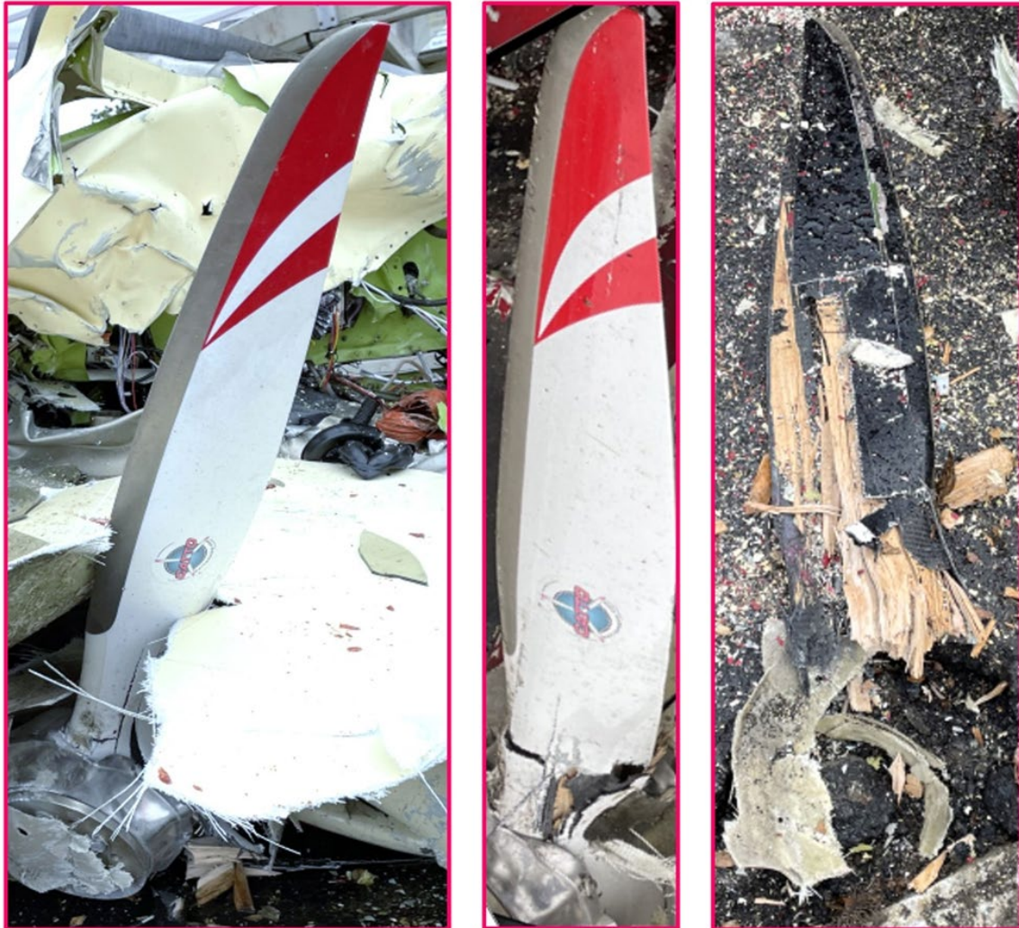
Figure 8: View of separated propeller blades.
