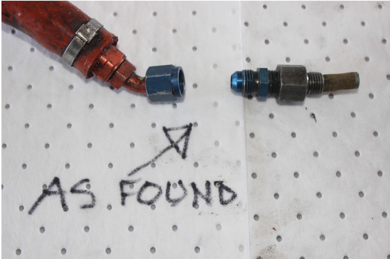
Photograph 7 - View of detached fuel line
