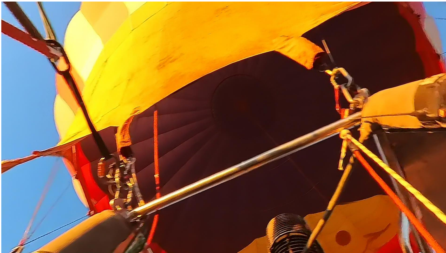
Figure 1. View at 01:54 in the second video, as the camera passed through the basket, showing the deflation system vent fully closed.
