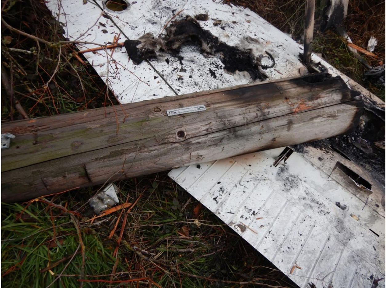
Figure 4. Middle section of the support pole rests on the underside of the right wing.
