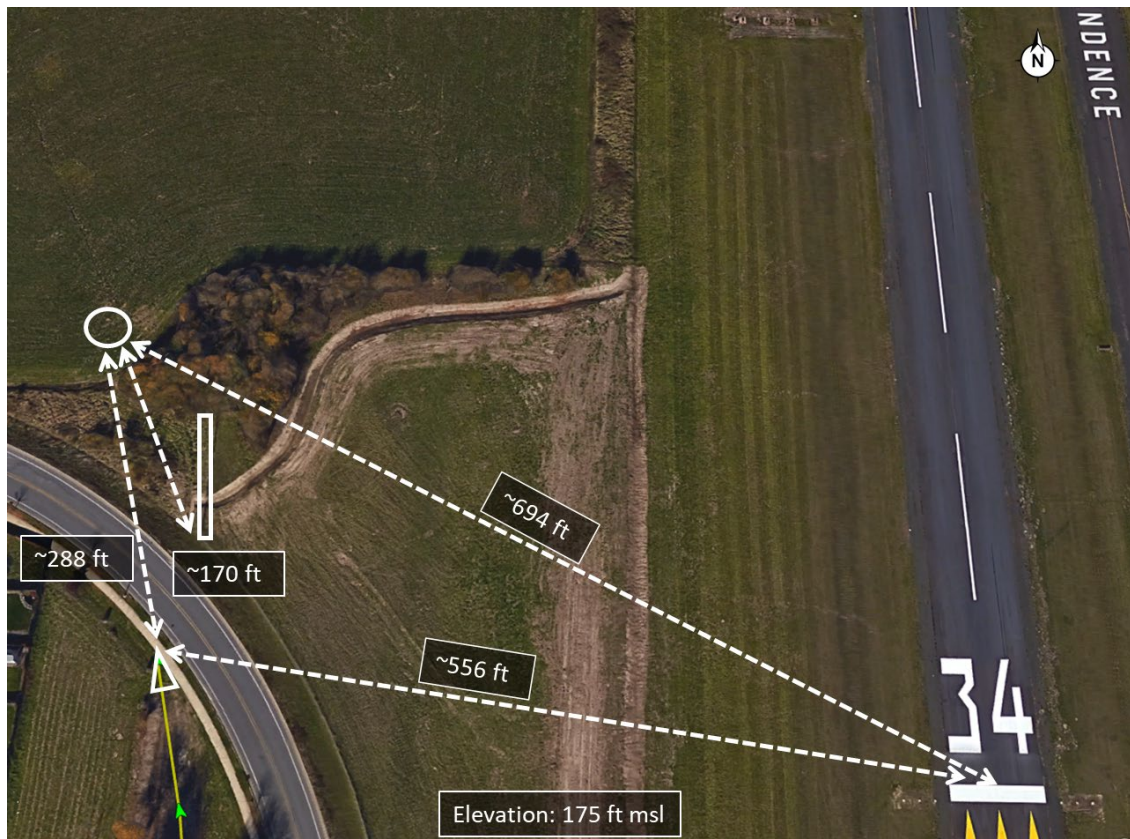
Figure 1. Image showing the last ADS-B point (triangle) open field, the support pole (rectangle) the runway and accident site (circle).
