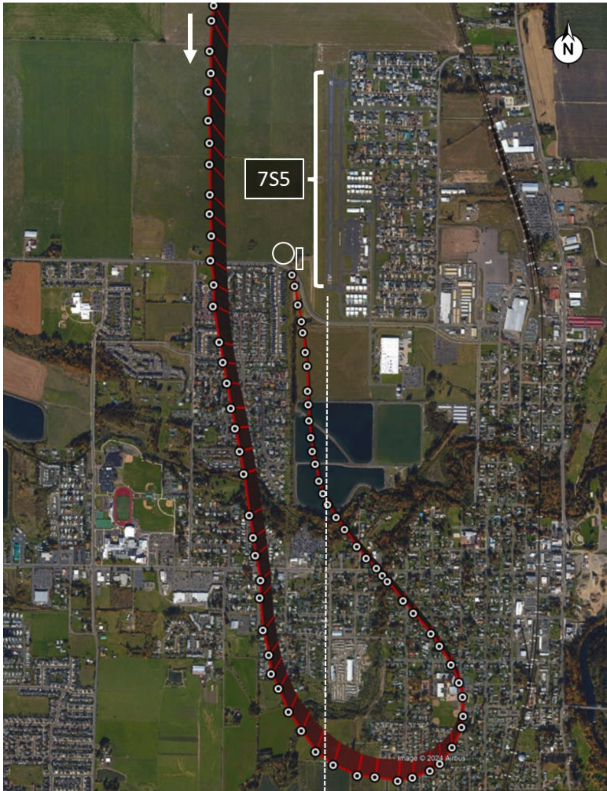
Figure 2. Image of the ADS-B flight track data and the runway centerline (dashed line). Arrow points to the direction of travel.
