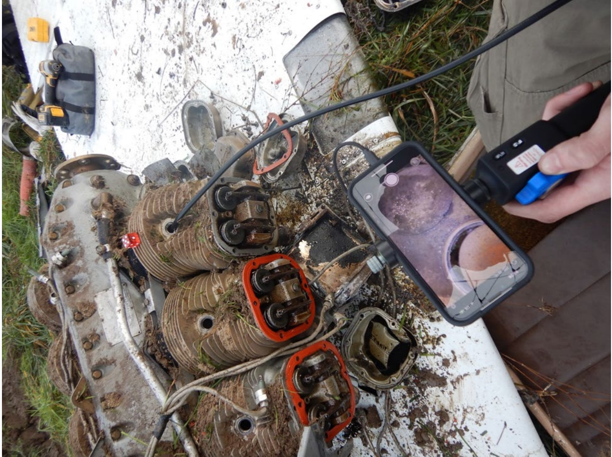
Figure 13. Borescope of the number 5-cylinder.
