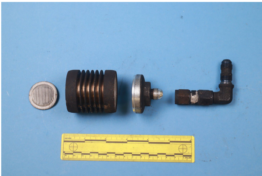
Figure 10. Photograph of the firewall elbow placed in series relative to the 10-micron fuel filter housing (disassembled) and the pleated filter element.
