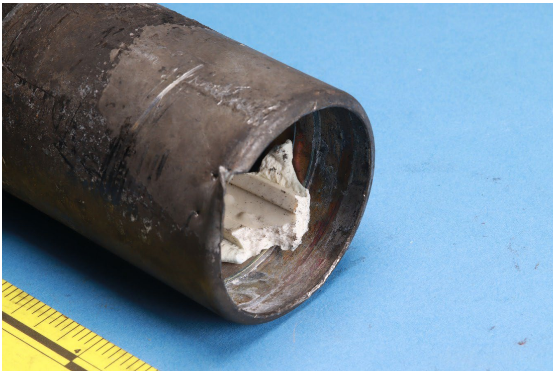
Figure 8. Photograph of one end of the electric fuel pump housing where a white material was observed inside the housing.
