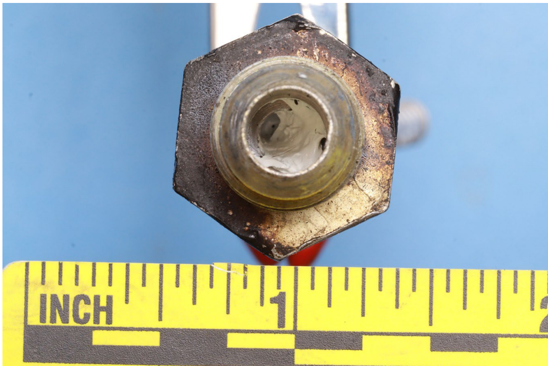
Figure 21. A view looking into the fitting of the servo filter element where a white material obstructed the interior of the fitting.
