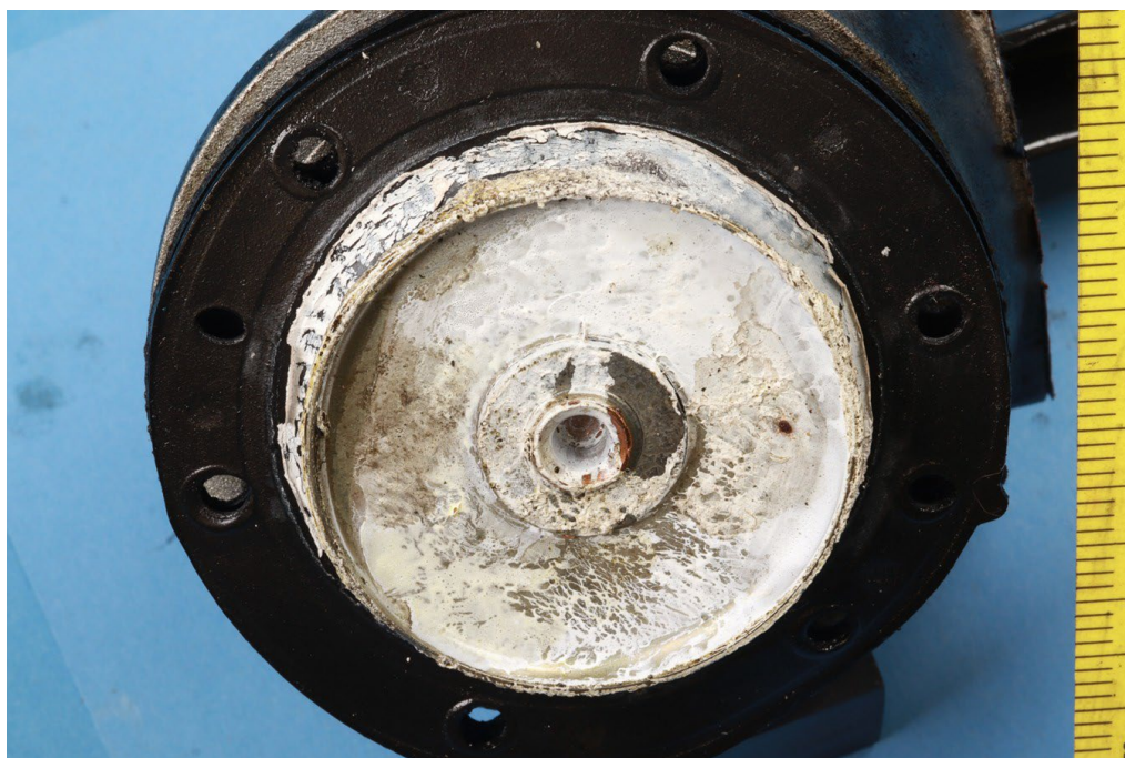
Figure 17. Photograph of the fuel pump body with the diaphragm seals as viewed from the pumping chamber side. A similar white material was observed covering the pumping chamber components.
