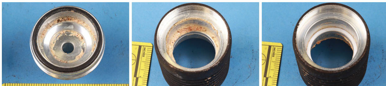
Figure 12. Photographs of the interior surfaces of the 10-micron fuel filter housing where off-white material deposits were observed.
