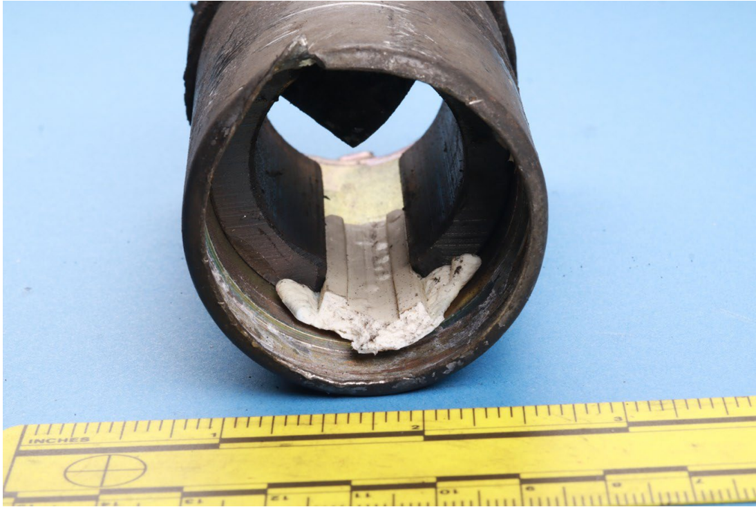
Figure 9. Photograph looking axially through the electric fuel pump housing showing another view of the white material observed between two curved plate magnets in the housing.
