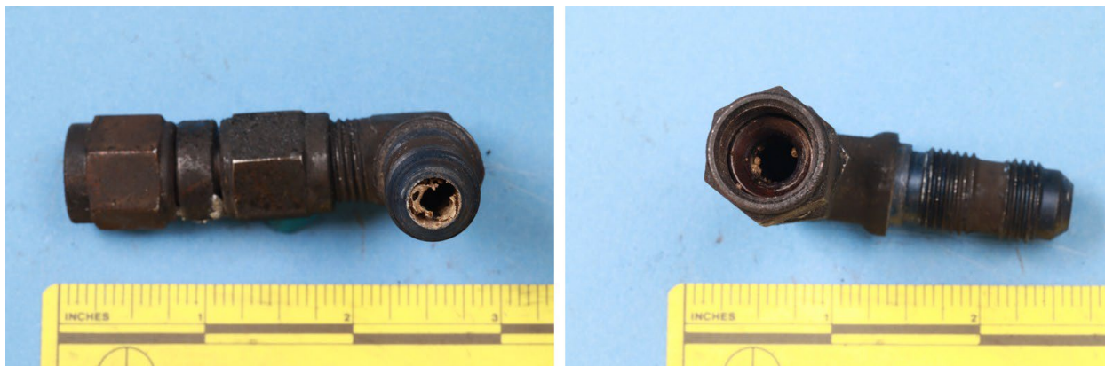
Figure 11. Closer views of each end of the firewall elbow fittings where tan material deposits were observed on the inner surfaces of the fittings.
