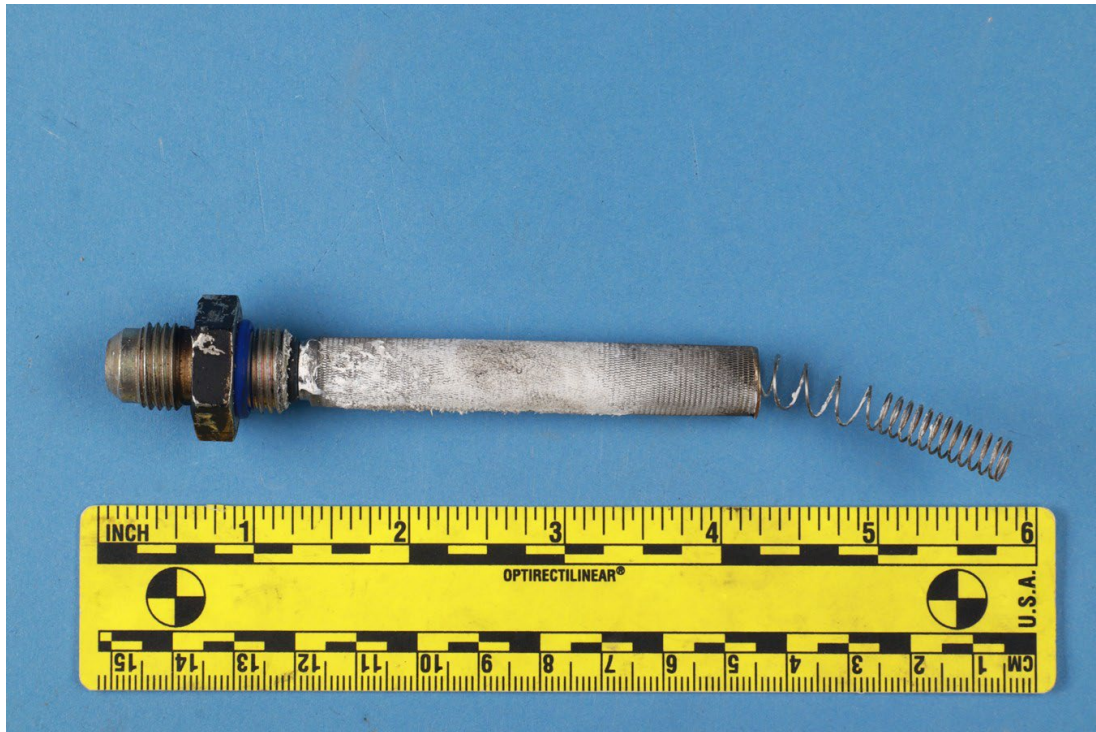
Figure 20. Photograph of the fuel injector servo filter where a white material was observed on and protruding from the filter screen element.
