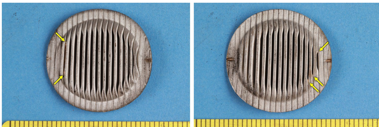
Figure 13. Photographs of each side of the 10-micron filter element where off-white material deposits were observed between filter pleats, examples of which are indicated by yellow arrows.
