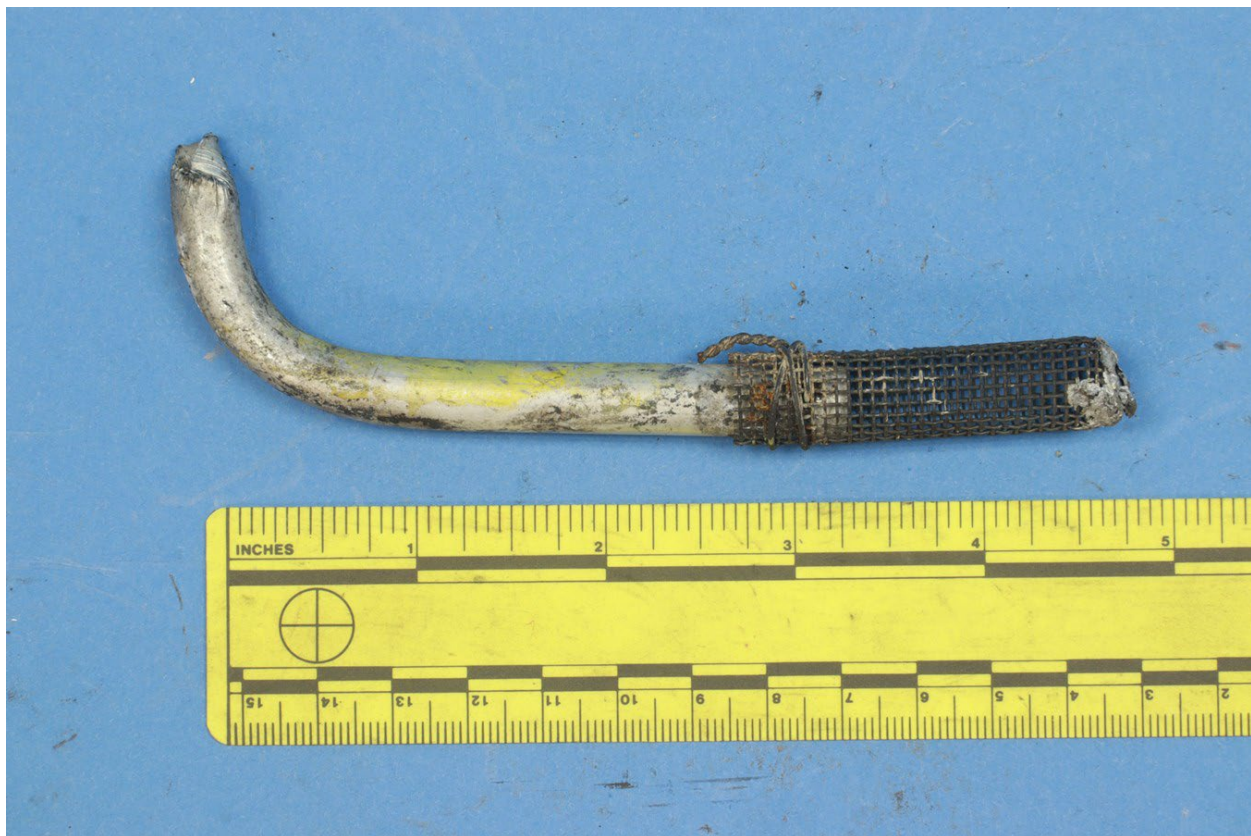
Figure 2. Photograph of the fuel tank pickup with attached screen which was fractured above the tubing bend. A deposit of molten metal was observed at the end of the screen.
