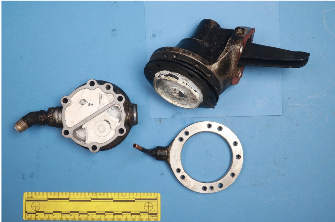
Figure 14. Photograph of the disassembled engine driven fuel pump.
