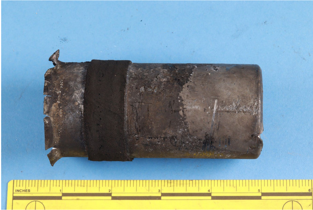
Figure 7. Photograph of the exterior of the electric fuel pump housing. Black soot deposits were observed covering the outer surface.
