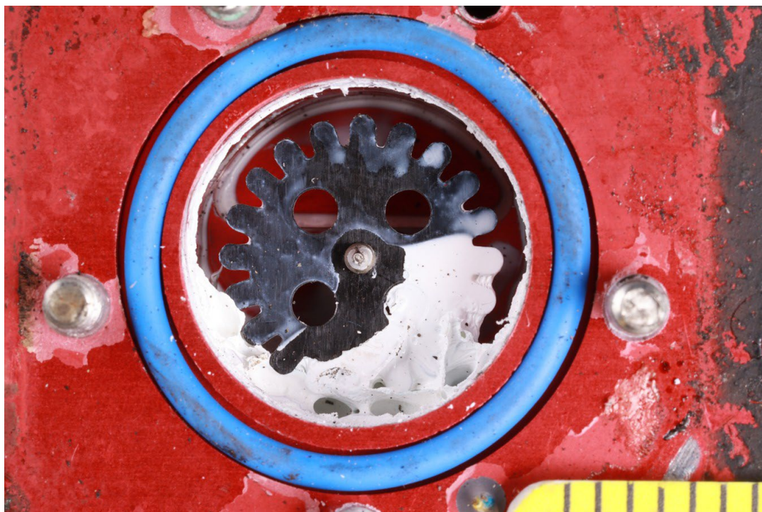
Figure 19. A closer view of the interior of the fuel flow transducer shown in the previous figure showing a black wheel component entangled in a white material.
