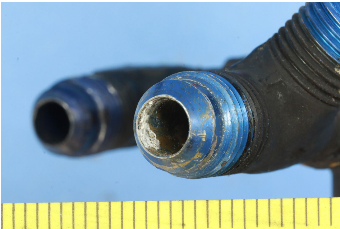
Figure 4. Closer view of the fuel selector fitting indicated in figure 3 where a white material deposit was observed on the inner surface of the fitting.
