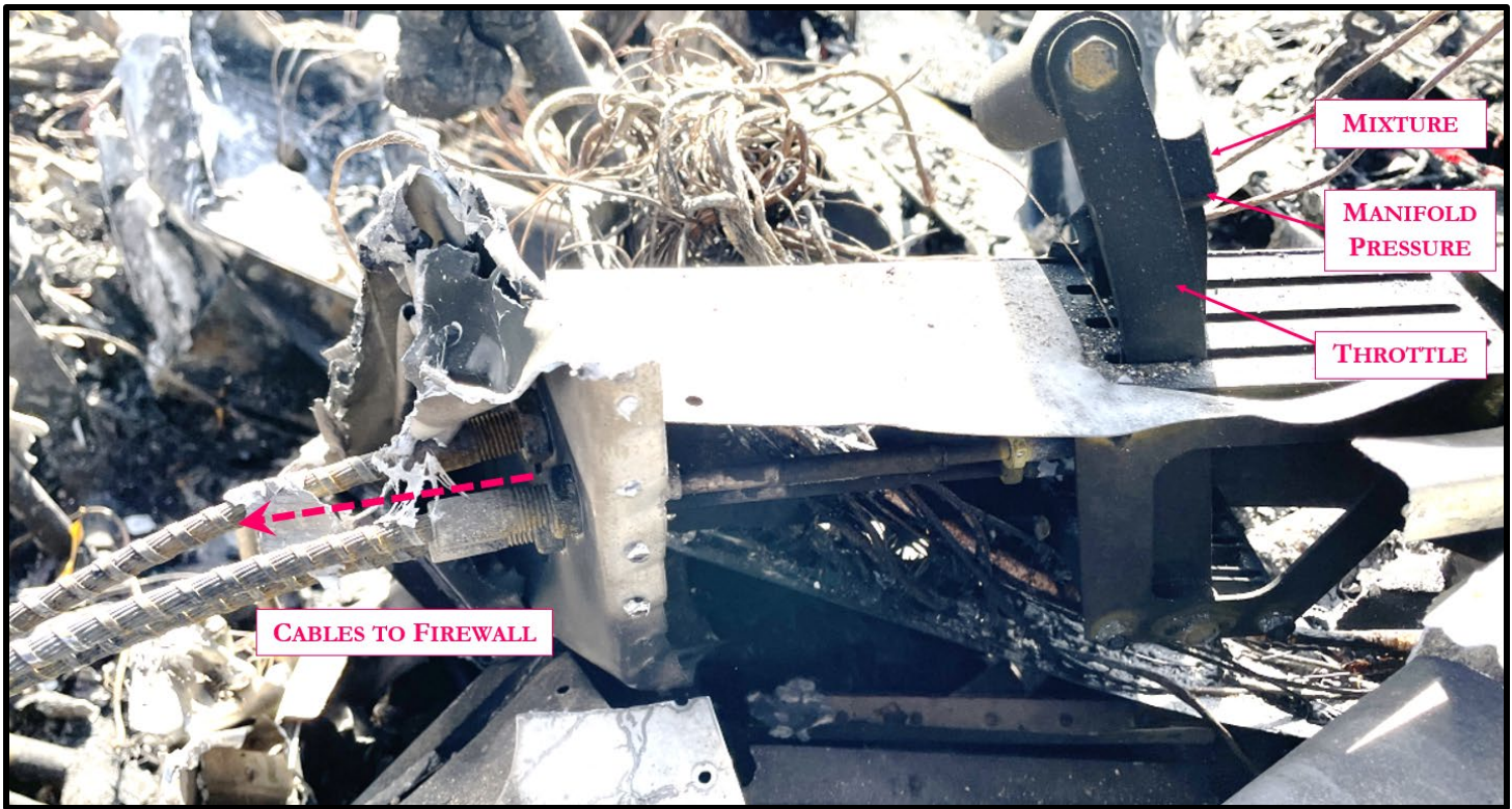
Figure 16: Throttle Quadrant Showing Cables Connect (showing left side)
