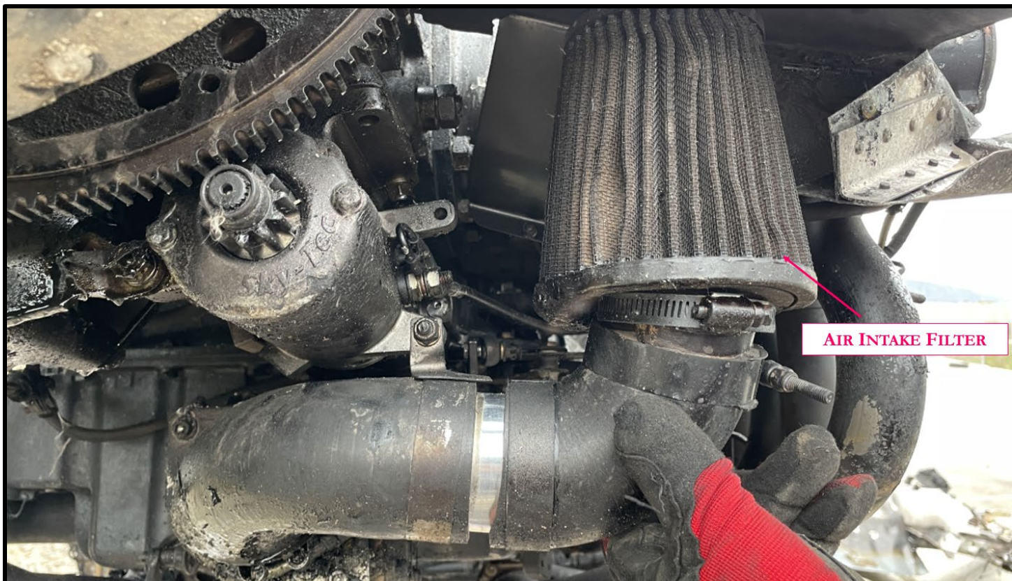
Figure 37: Air Intake Filter
