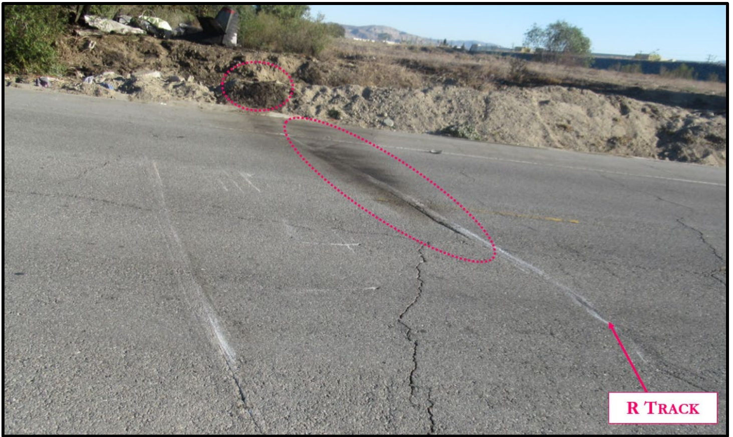
Figure 10: Black Residue Near the Right Track and the Darkened Berm
