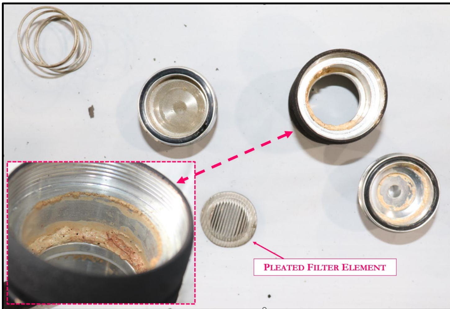
Figure 28: Inside Firewall Fuel-Filter
