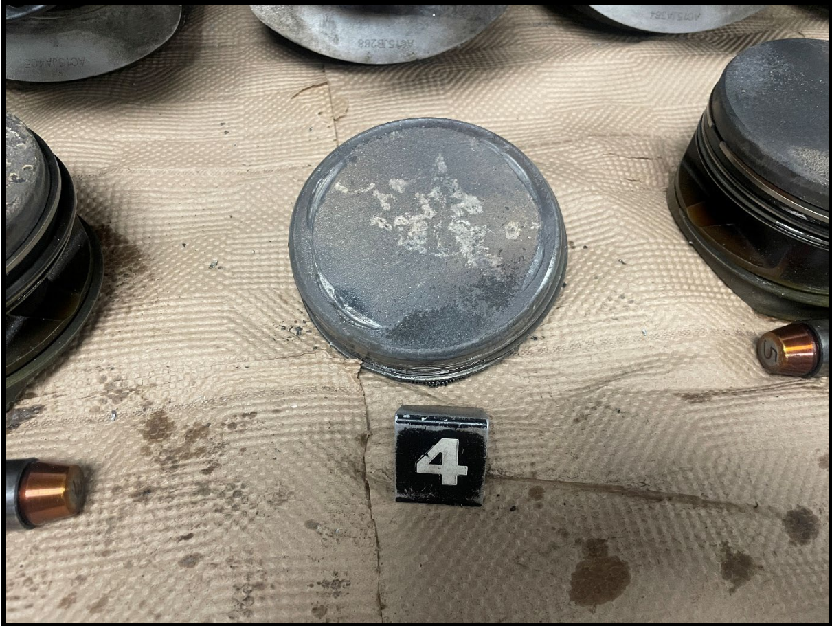
Figure 6: View of the remaining No. 4 cylinder piston
