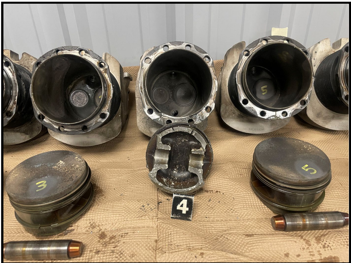
Figure 5: View of No. 4 cylinder removed from crankcase and its associated piston
