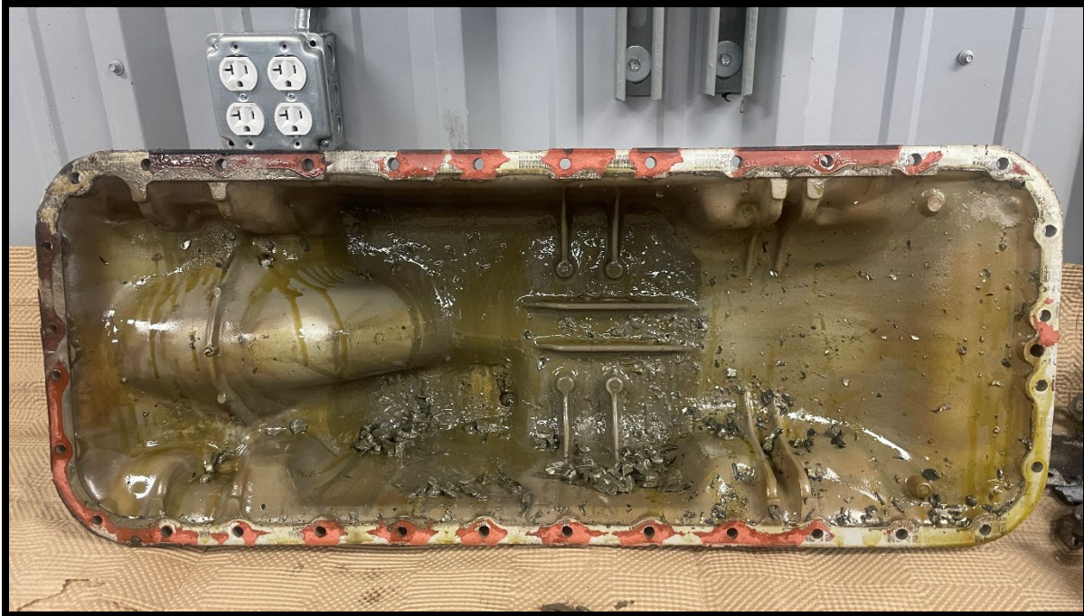
Figure 4: View of metallic debris in the oil sump
