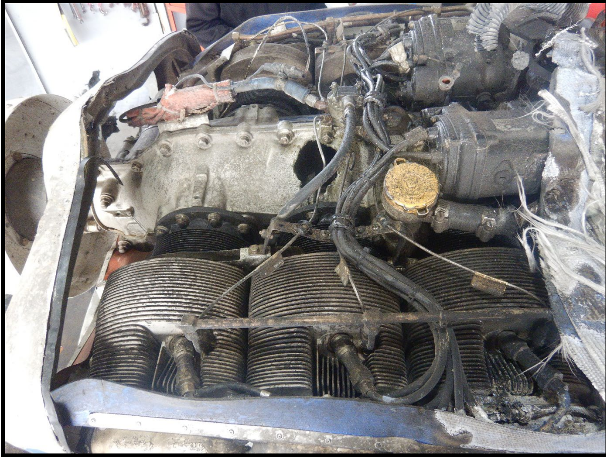
Figure 2: Top view of the crankcase with a 2.5-inch x 2-inch hole above No. 4 cylinder
