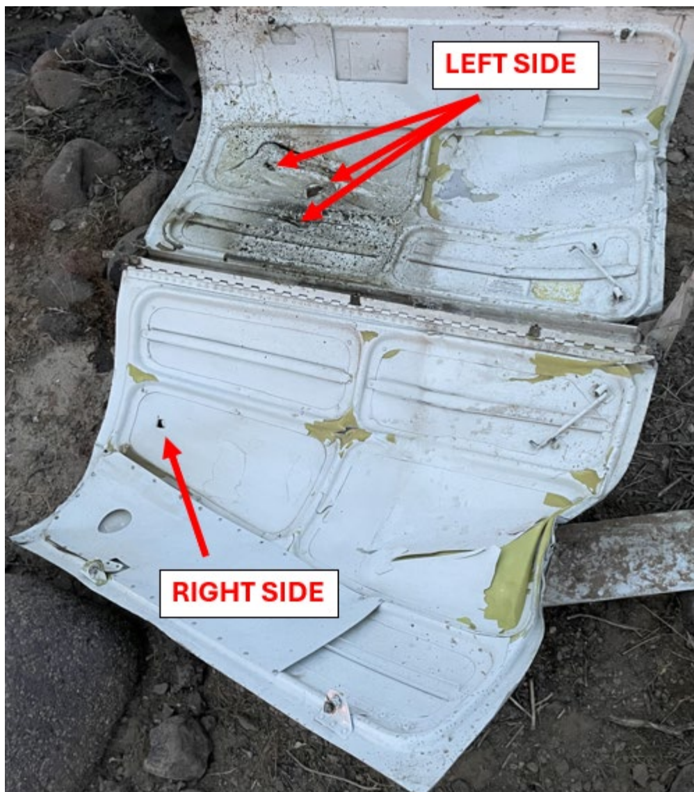
Figure 3: View of the left and right upper engine cowling protrusions
