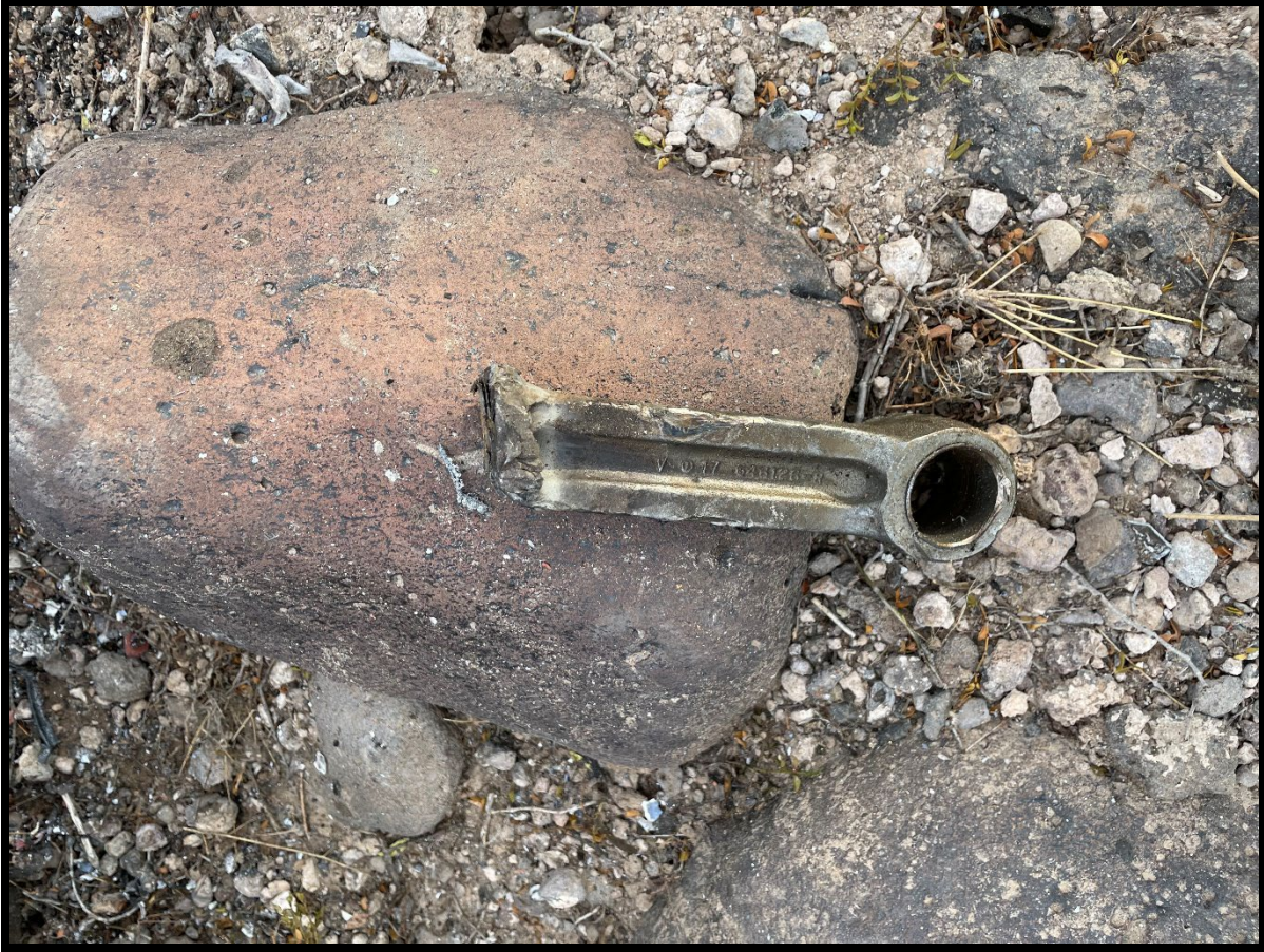
Figure 7: View of No. 4 piston connecting rod at the accident site
