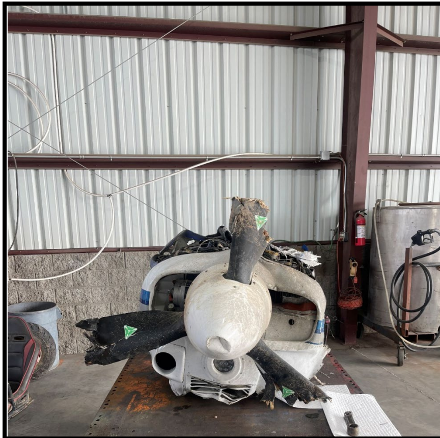
Figure 9: View of impact damage to propeller blades and spinner
