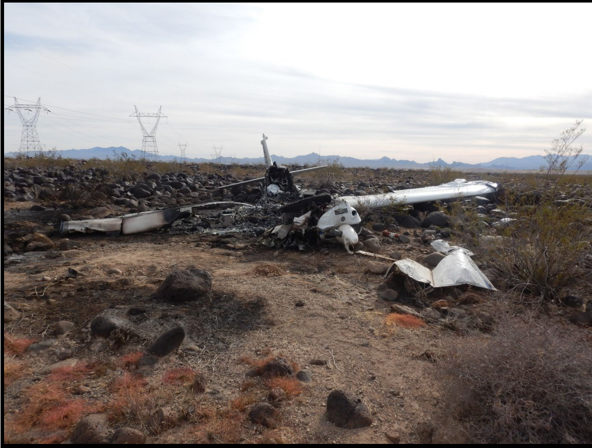
Figure 1: North to south view of high-tension powerline wires, and a forward-to-aft view of the airplane with thermal and impact damage sustained
