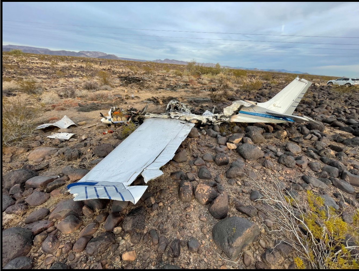
Figure 5: View of high-tension powerline wires, along with the thermal and impact damage sustained to the left side of N4171S
