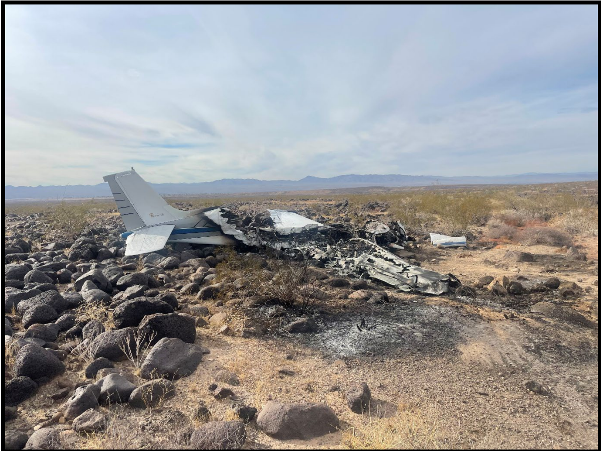
Figure 4: View of the impact and thermal damage sustained to the right side of the N4171S
