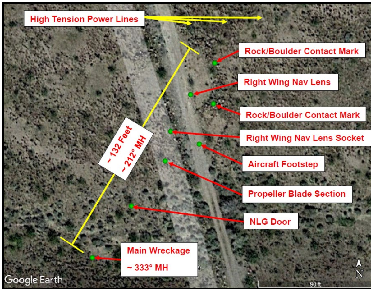
Figure 3: Wreckage and debris path diagram
