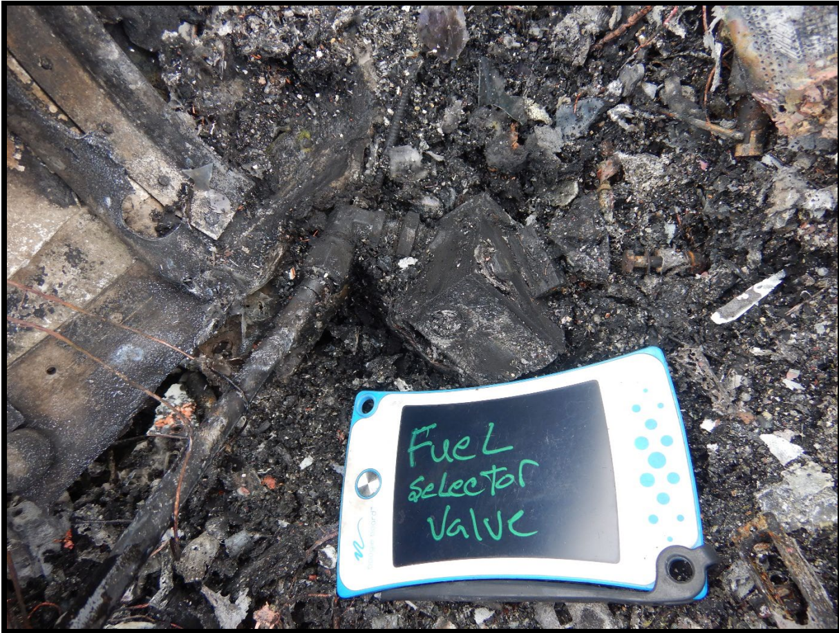
Figure 6: Fuel selector in the Off position
