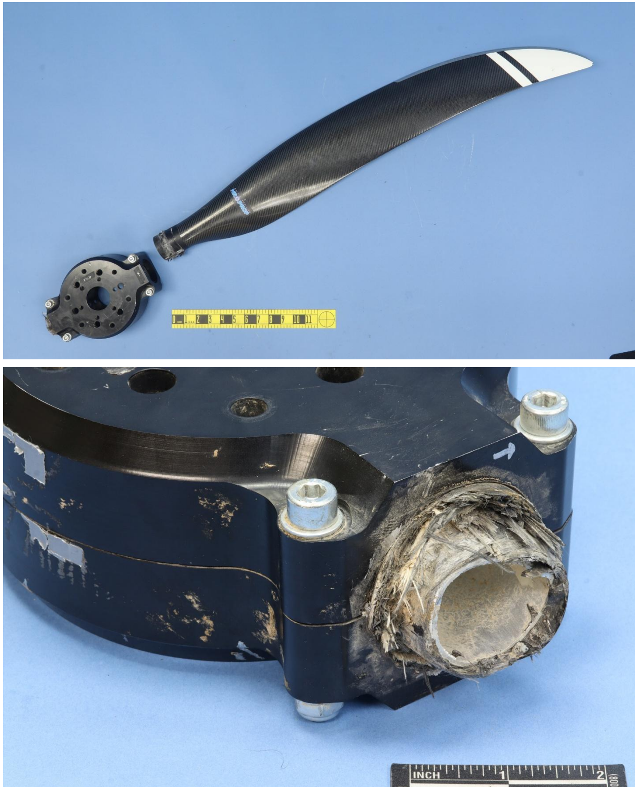
Figure 1. Top image: Overview of propeller hub with retained blade root and separated blade. Bottom image: The retained root of the separated blade.
