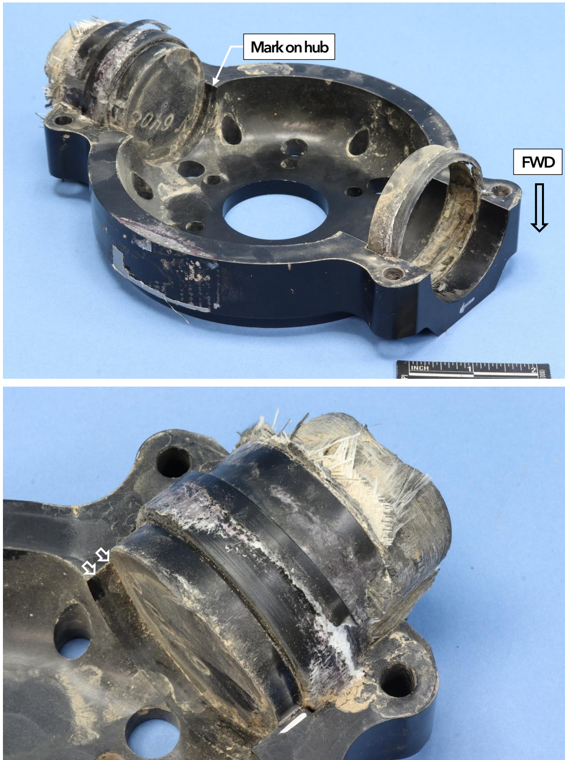
Figure 10. Upper image: Overview of hub with aft half removed. Lower image: Closer image of retained blade root. Arrows indicate the location of a mark on the hub and the position of the blade root.
