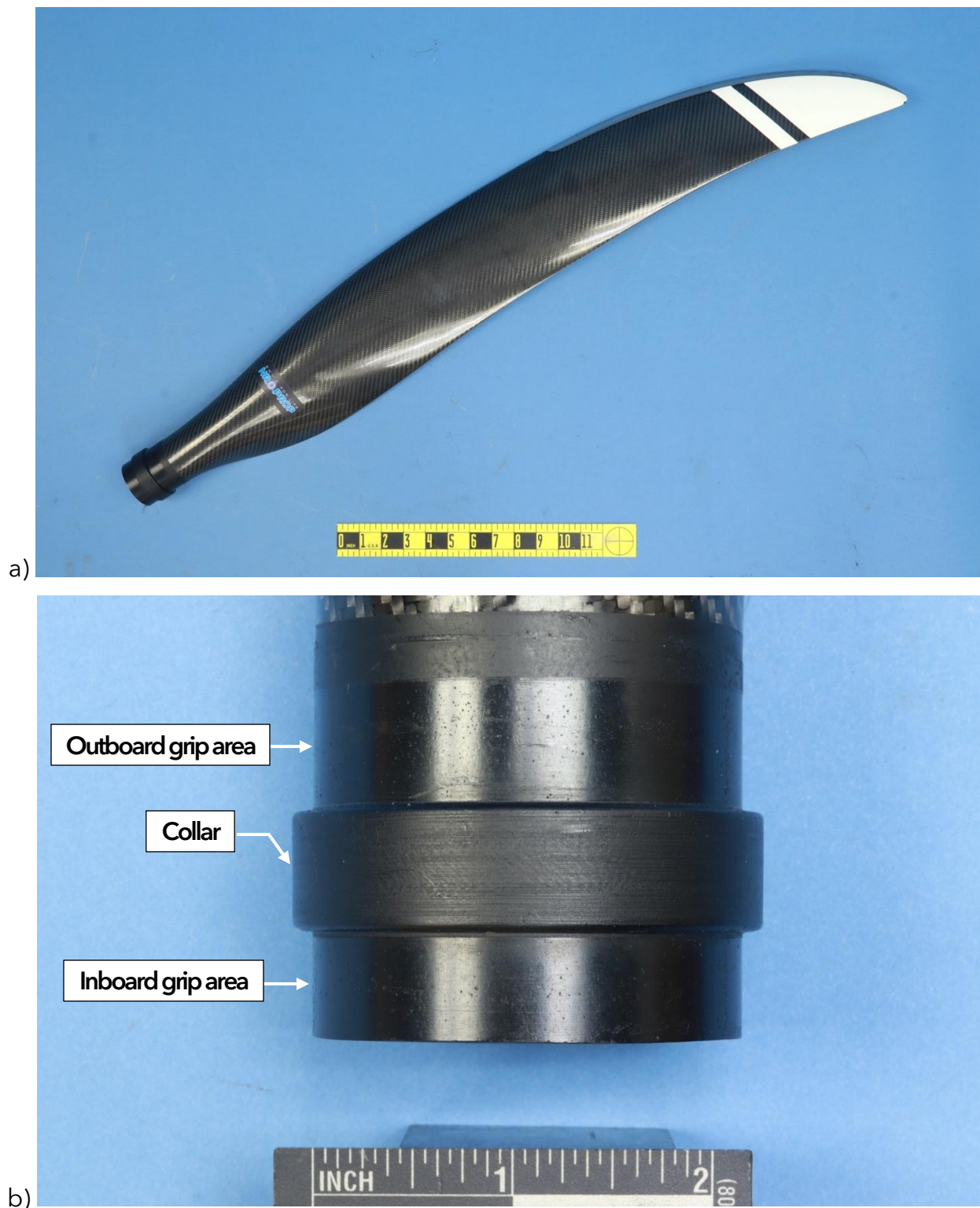
Figure 2. Exemplar propeller blade: a) Overview image and b) blade root.
