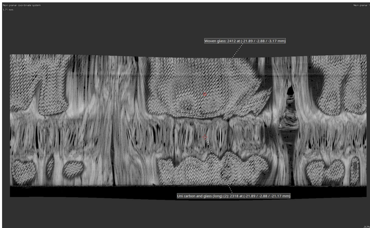
Figure 19. CT image of the exemplar propeller blade root - woven glass layers unrolled.
