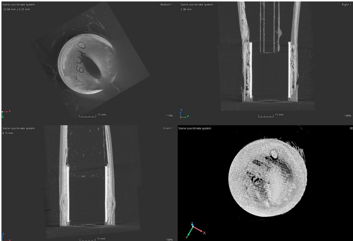
Figure 24. CT images of the accident propeller blade root showing SN 6410 at the blade butt.
