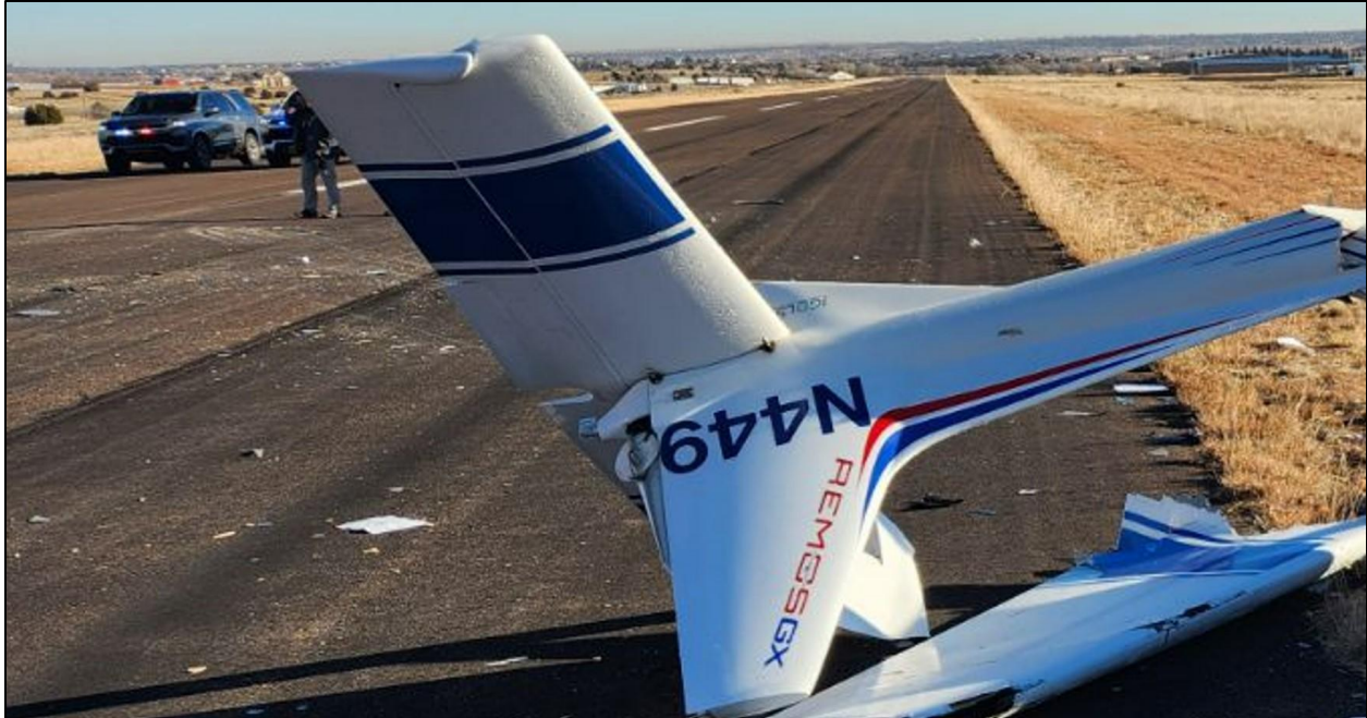
Figure 2-Accident site, photo zoomed in to show frost covering the top side of the horizontal stabilizers. (Courtesy of the Airport Manager)
