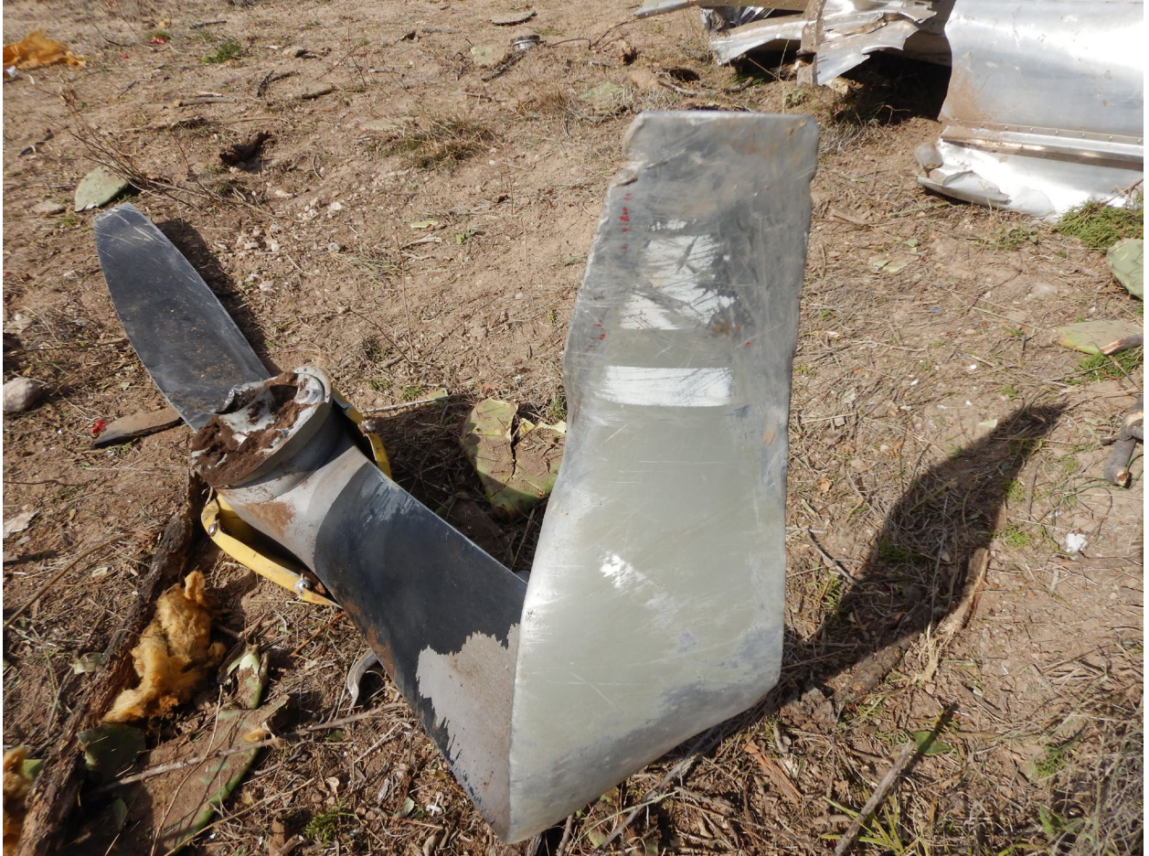
Figure 20. Propeller, forward view at bent tip.
