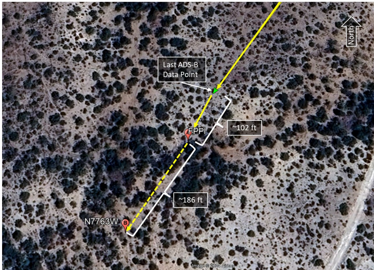
Figure 3. Google Earth image showing the location of the last ADS-B data point, the FPPI, and the airplane wreckage.
