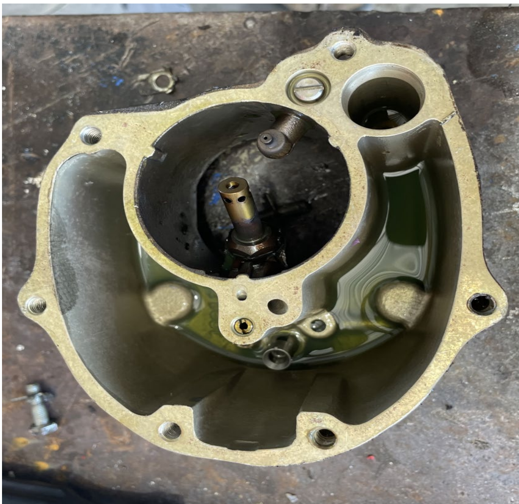
Photograph 9 - View of Carburetor Bowl
