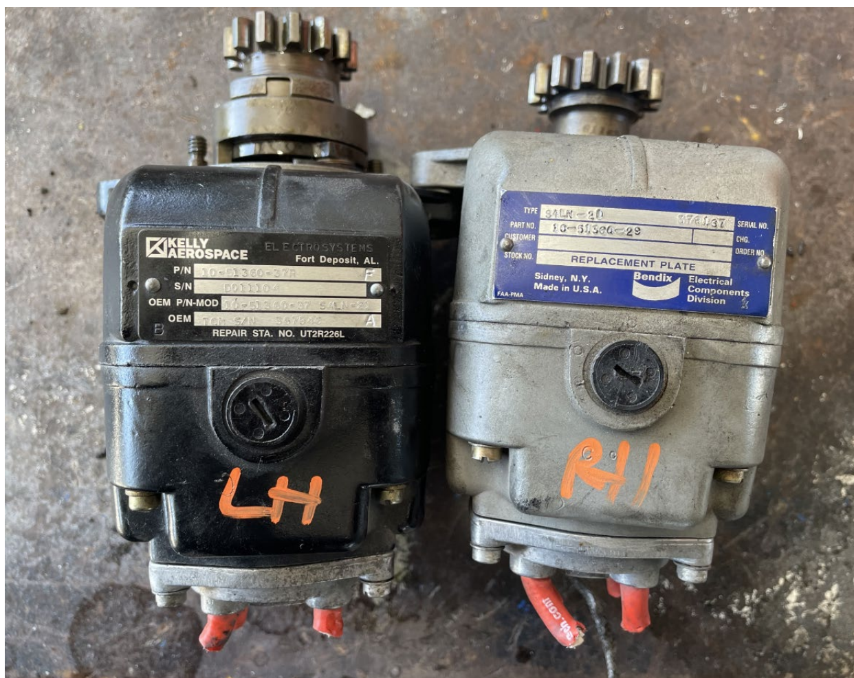
Photograph 8 - View of removed magnetos
