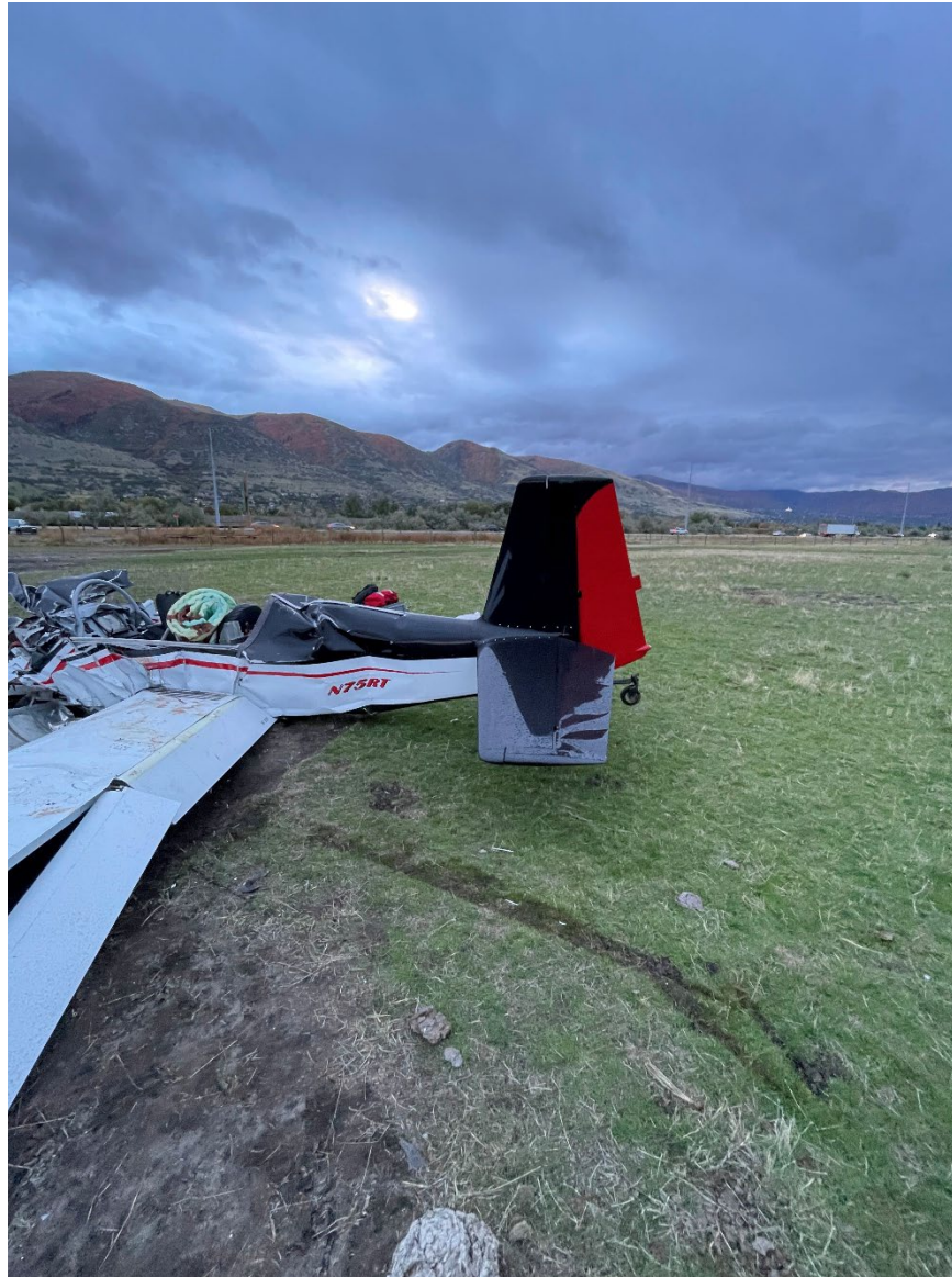
Photograph 3 - View of ground scars and resting position of the airplane
