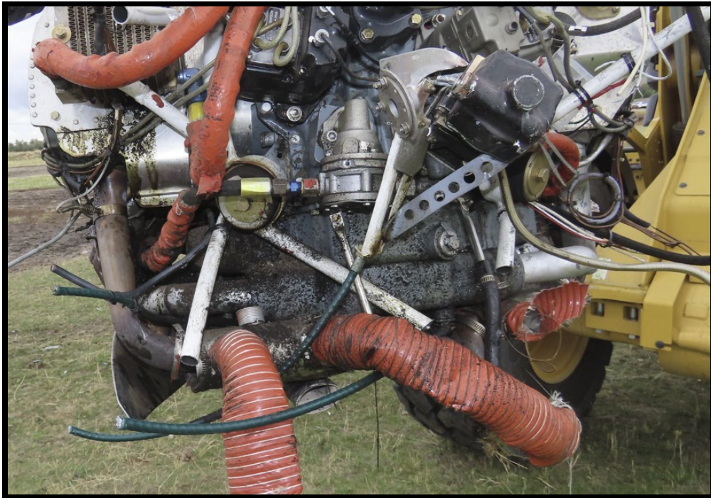
Figure 10: View of residual oil and dirt accumulation on the engine
