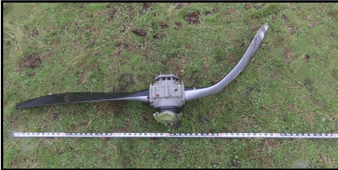
Figure 8: View of propeller blade damage
