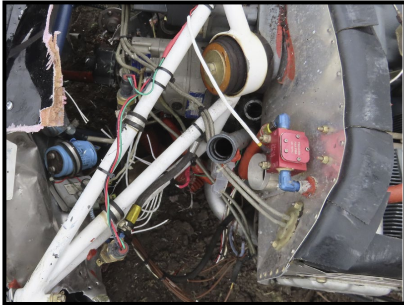
Figure 1: View of damaged oil filler neck
