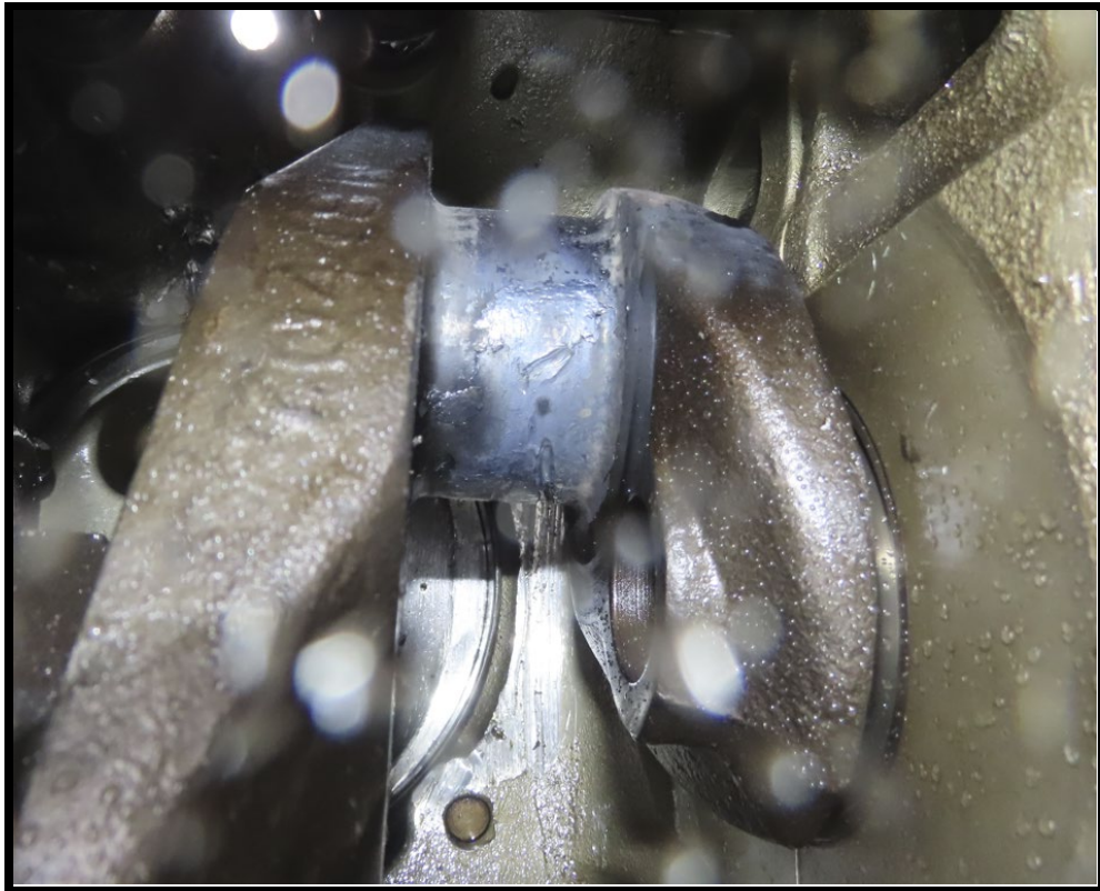
Figure 7: View of oil starvation signatures on crankshaft journal
