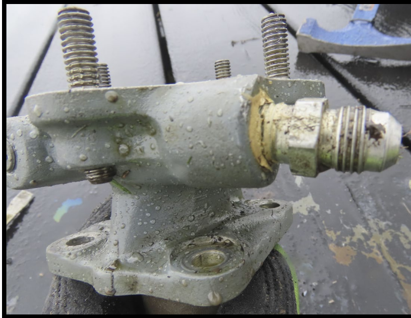
Figure 11: View of hairline cracks throughout the propeller governor mounting adapter
